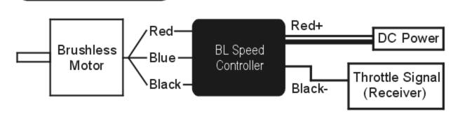
Exchange two wire for changing motor rotation direction.
