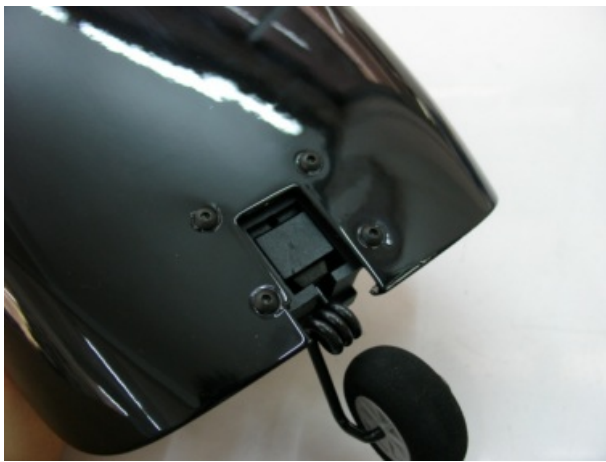
MOUNT THE NOSE LANDING GEAR WITH 3 X 10 MM ROUND SOCKET HEAD SCREWS AND LOCK NUTS.
