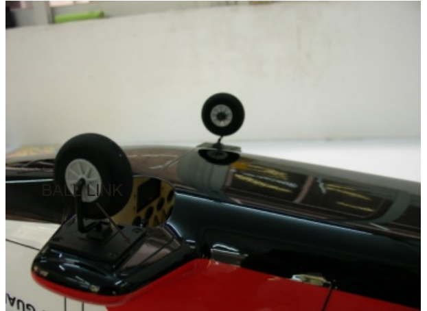
MOUNT THE NOSE LANDING GEAR WITH 3 X 10 MM ROUND SOCKET HEAD SCREWS AND LOCK NUTS.
