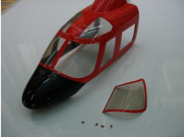
ONE SIDE OF WINDSHIELD IS REMOVEABLE FOR BATTERY REPLACEMENT. IT IS FASTENED BY 4 PC. OF 3 X 6 TAPPING SCREWS WITH 10x10x1.5 PLYWOOD.
