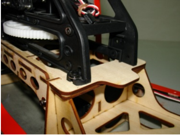
FASTEN MECHANISM BY 3x12 SOCKET HEAD SCREWS WITH WASHER IN FRONT
