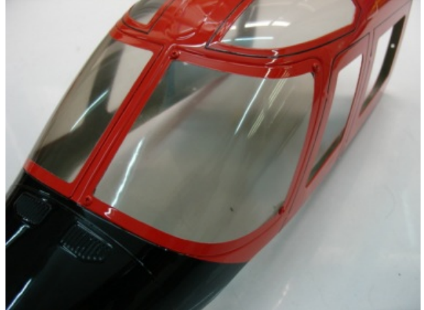
ONE SIDE OF WINDSHIELD IS REMOVEABLE FOR BATTERY REPLACEMENT. IT IS FASTENED BY 4 PC. OF 3 X 6 TAPPING SCREWS WITH 10x10x1.5 PLYWOOD.
