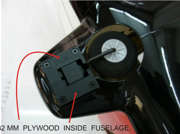
MOUNT THE MAIN LANDING GEAR WITH 2.6 X 12 MM FLAT HEAD TAPPING SCREW.
