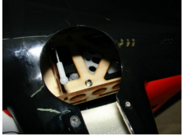
FASTEN MECHANISM BY 3x12 SOCKET HEAD SCREWS WITH LOCK NUT UNDER PLYWOOD PLATFORM IN REAR
