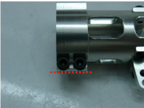
CUT TAIL GEAR BOX AS SHOWN
