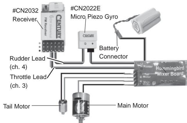
2. Press the tail motor and main motor connectors to the board, note that the two red wires are beside each other when connected to the board.
