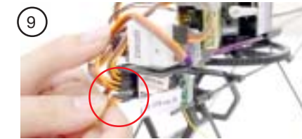
9. For CP Hummingbird plug 3rd servo (collective pitch) into channel 6.
