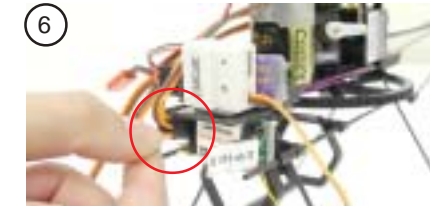
6. Plug in channel 3 for throttle (mixer board).
