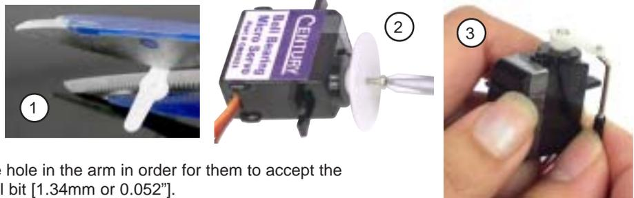
3. Some servo arms require widening the hole in the arm in order for them to accept the Hummingbird's pushrods using a #55 drill bit [1.34mm or 0.052"].
