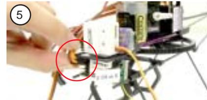
5. Plug in channel 2 for elevator servo.
