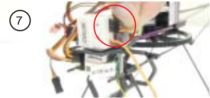
7. Plug mixer rudder lead into gyro (signal wires must face each other).
