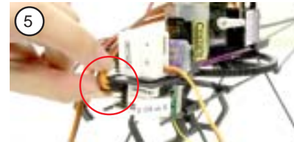
5. Plug in channel 2 for elevator servo.
