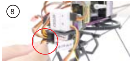
8. Plug gyro into channel 4 for rudder.
