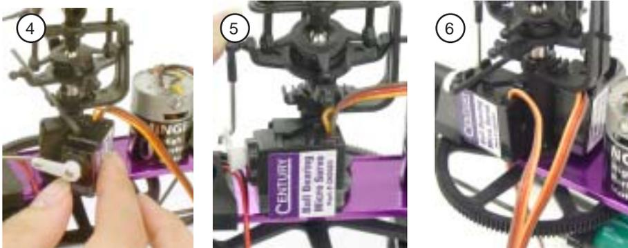
4. Once the mounting position of the servo is determined carefully mount the servo to the mast tower. If the servo has a label on the same side that will mount with double sided tape, peel off the label and clean the surface using rubbing alcohol.
