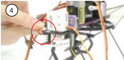
4. Plug in channel 1 for aileron servo.
