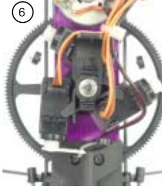
4. If the servo has a label on the same side that will mount with servo tape, peel off the label and clean the surface using rubbing alcohol. Once the mounting position of the servo is determined carefully mount the servo to the mast tower.
