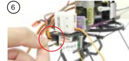
6. Plug in channel 3 for throttle (mixer board).
