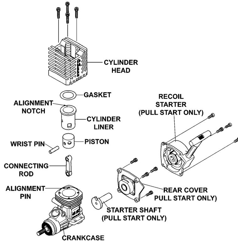
**How to install your new DuraTrax piston/cylinder assembly into your O.S.® Max® .12 Series R/C engine:**
