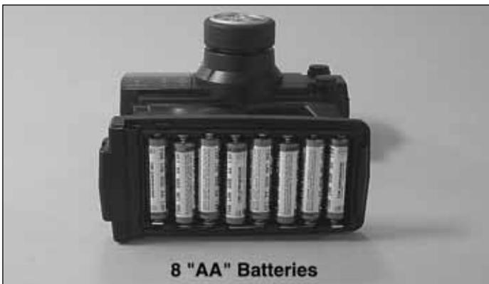
❑ 2. Slide open the battery door on the bottom of the transmitter. Install eight (8) "AA" batteries into the transmitter in the configuration molded into the plastic on the battery holder. Re-install the battery door.
