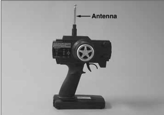
❑ 1. Install the transmitter antenna by screwing it into the hole on the top of the transmitter. **Note: After installing the antenna, give it a good tug to make sure it is properly installed.**
