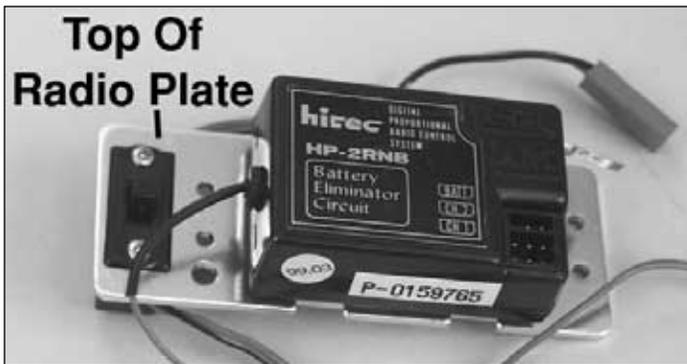
4. Attach the switch from your radio system so it is above the top of the radio plate (make sure the switch is in the OFF position). Remove the two screws on the top of the switch. Place the switch plate on top of the radio tray, the switch body on the bottom of the radio tray and then reinsert the screws from the top.
