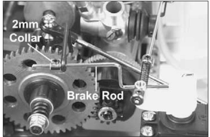
❑ 6. Install a 2mm collar at the end of the brake rod and another 2mm collar at the end of the throttle rod. Place a small amount of thread locking compound on two of the (3) 3 x 3mm set screws and thread them into the 2mm collars. Do not tighten the set screws all the way. In the next section we will make adjustments to the collars.
