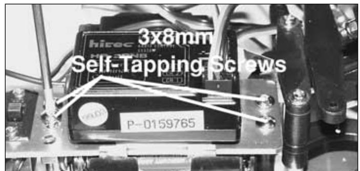
8. Attach the radio tray to the radio tray posts with (4) 3 x 8mm self-tapping screws.
