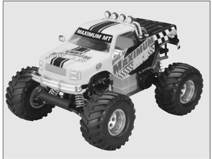
16. Remove the body clips from the parts bag. Place the body on the body mounts. On each body mount place a body clip.
