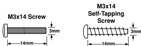
The illustration above shows how to identify the types of screws used throughout this instruction manual.
