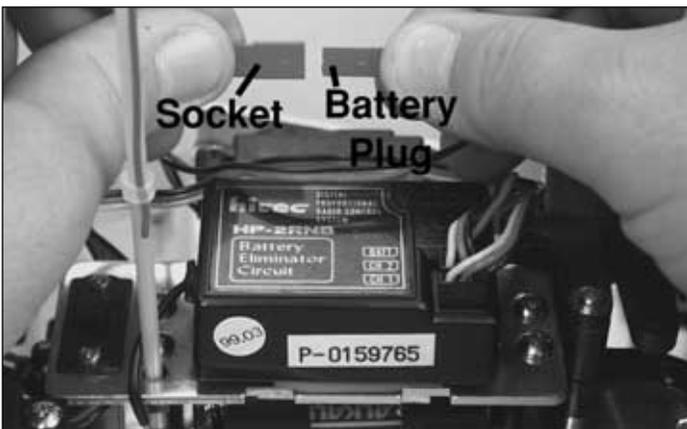
❑ 7. Re-install the receiver battery holder under the radio plate. Make sure that the receiver switch is in the off position. Plug the connector on the receiver battery into the socket on the receiver switch. Tuck the wires between the servo and receiver battery so they will not get caught on anything.
