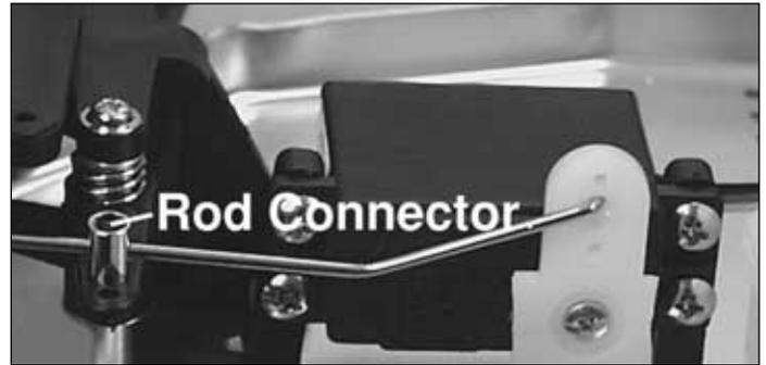
❑ 8. Slip the steering rod through the hole in the rod connector that is already installed on the servo saver. (Use the screw that came with your radio system to attach the servo arm to the steering servo.) Do not tighten the set screw on the rod connector. You will make the steering adjustments later.
