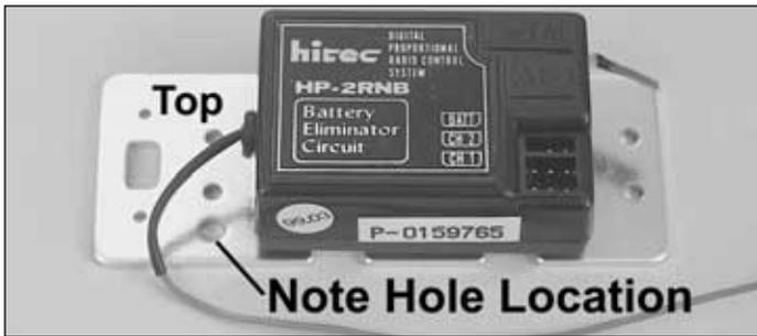
3. Using the provided double-sided tape, attach the radio receiver to the top of the radio tray. To find the top of the radio tray, place the large circular hole to the lower left as shown. Make sure that the receiver is installed in the space between the sets of screw holes as shown above.
