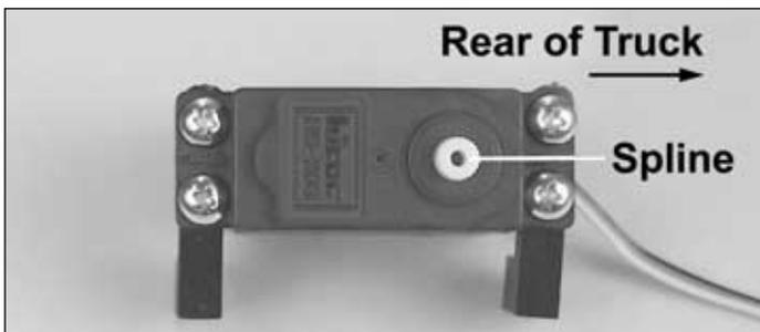
2. Attach the servo mounts to the steering servo with (4) 3 x 8mm self-tapping screws. Note that the servo spline will mount towards the rear of the truck.
