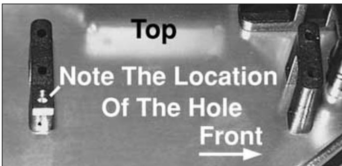
5. Attach the radio tray mounts as shown to the chassis with (4) 3 x 8mm self-tapping screws.
