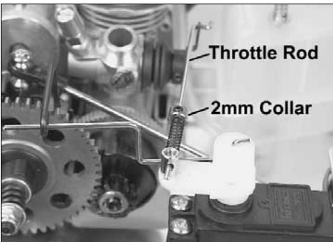
❑ 5. Insert the throttle rod into the outer hole in the carburetor arm. Assemble in order, a 2mm collar and the throttle spring. Next insert the throttle rod through the rod connector on the throttle servo.
