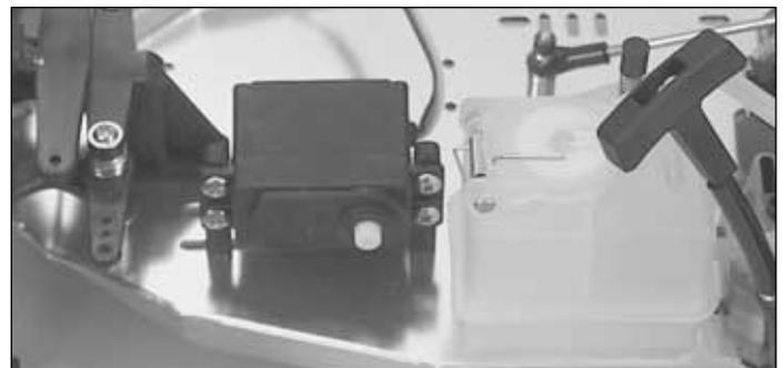
3. Attach the steering servo assembly to the chassis with (4) 3 x 8mm self-tapping screws in the holes provided as shown above.
