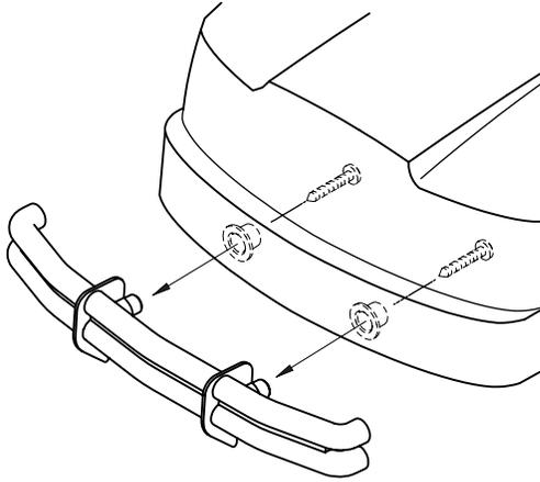
❑ 5. Drill two 1/4" (6mm) holes in front of body using the molded-in dimples as guides. Install the front brush guard as shown with two 2.6 x 6mm self-tapping screws and the collars included.
