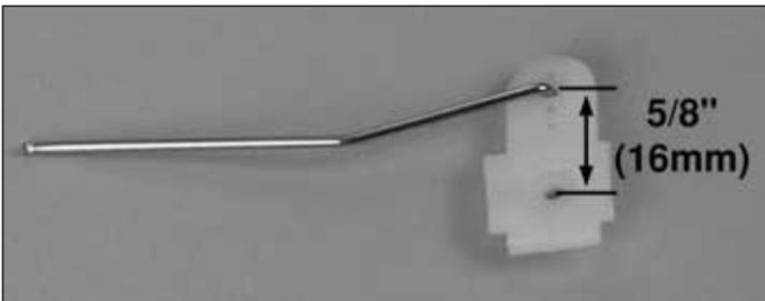
❑ 6. Put the steering rod into the third hole from the center of the servo arm (approximately 5/8" or 16mm). You may need to enlarge the hole in the servo arm with a 5/64" (2mm) drill or a hobby knife.
