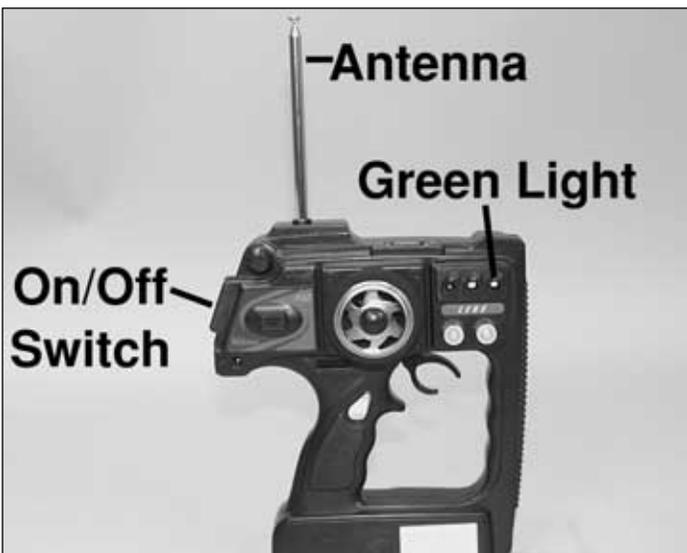
❑ 8. Remove the transmitter antenna from the holder and screw it into the hole on top of the transmitter.
