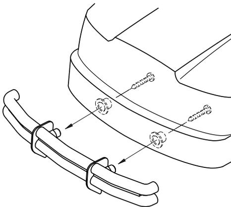
14. Drill two 1/4" (6mm) holes in front of body using the molded-in dimples as guides. Install the front brush guard as shown with two 2.6 x 6mm self-tapping screws and the collars included.
