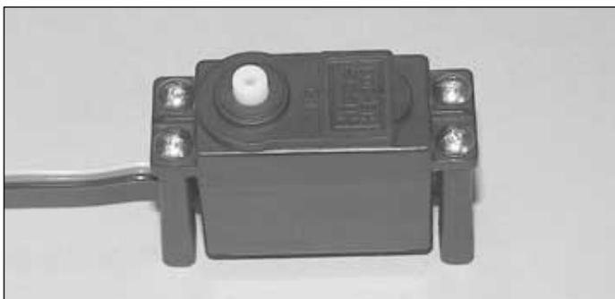
❑ 2. Use the (4) 3 x 8mm self-tapping screws to attach the throttle servo to the throttle servo mounts.
