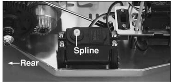
❑ 3. Use the (4) 3 x 8mm self-tapping screws to attach the throttle servo and the mounts to the chassis. Make sure that the servo spline is towards the rear.
