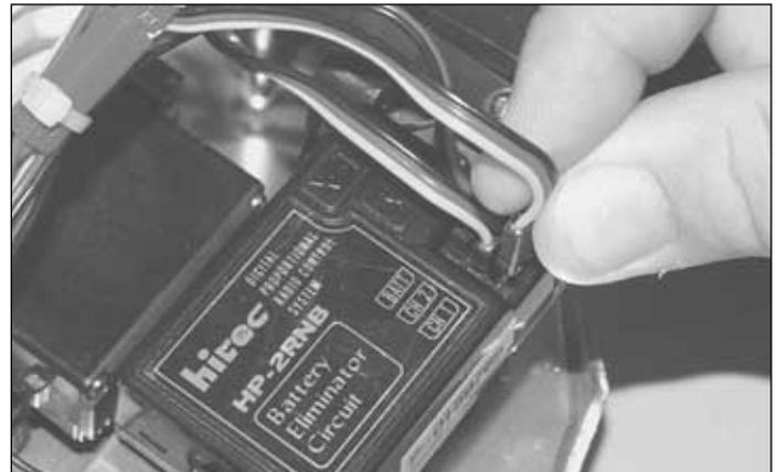
7. Plug the steering servo, throttle servo, and switch into the receiver. See your radio instructions to determine which channel is steering and which channel is throttle. The receiver switch plugs into the socket labeled "Battery," "Batt," or "B."
