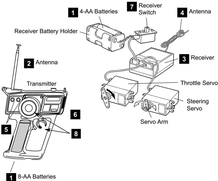
1. Install the batteries in the transmitter and the receiver battery holders.
