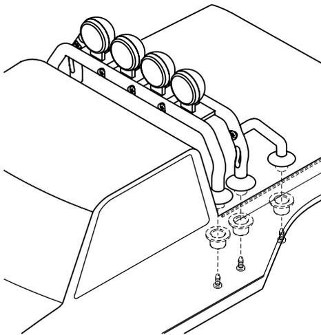
13. Drill six 1/4" (6mm) holes in the body using the molded-in dimples as guides. Install the rollbar onto body as shown using six 2.6 x 6mm self-tapping screws and the included collars.
