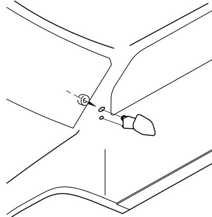
15. Drill one 1/8" (3mm) hole in each side of the body using the molded-in dimple as a guide, and one 5/64" (2mm) hole 7/16" (11mm) below and 7/16" back from first hole (use the pegs on the mirror as a guide). Install the mirrors as shown with the collars provided.
