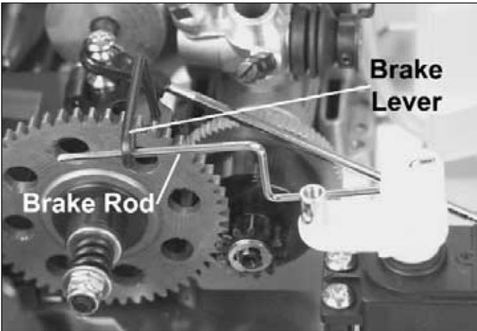
❑ 4. Place the servo arm on the throttle servo as shown in the photo above and place the brake rod through the brake lever. Do not install the servo arm screw yet. You will need to make adjustments before running your truck.
