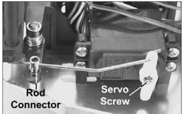
A) Remove the arm from the steering servo and re-install the arm facing straight up (see photo above).
