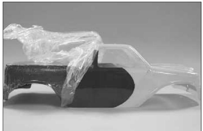
❑ 11. Remove the plastic from the outside of the body. Apply the decals if desired. For decal placement, see the photos on the box top.
