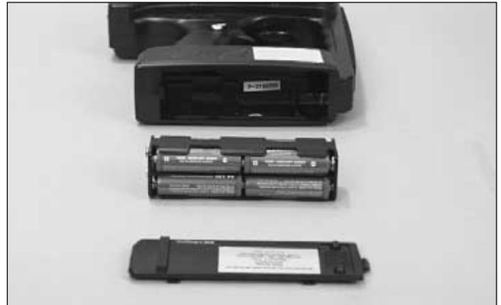
❑ 9. Slide open the battery door on the bottom of the transmitter and remove the transmitter battery holder. Place 8 "AA" batteries into the holder in the configuration molded into the plastic on the battery holder. Re-install the transmitter battery holder into the transmitter and re-install the battery door.
