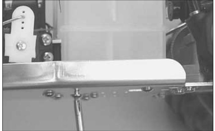
1. Remove the fuel tank by taking out the two screws on the bottom of the chassis.
