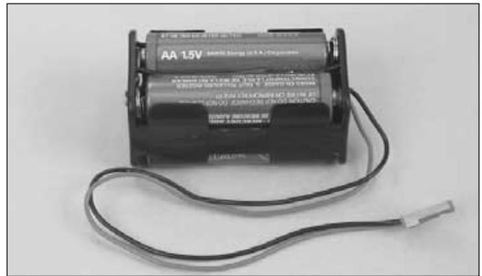
6. Remove from your radio system the 4-cell receiver battery holder and install (4) "AA" batteries (not included). The negative sides of the batteries are placed against the springs in the battery holder. Plug the connector on the receiver battery holder into the connector on the switch. Make sure the switch is in the OFF position. Place the receiver battery holder between the radio plate posts.
