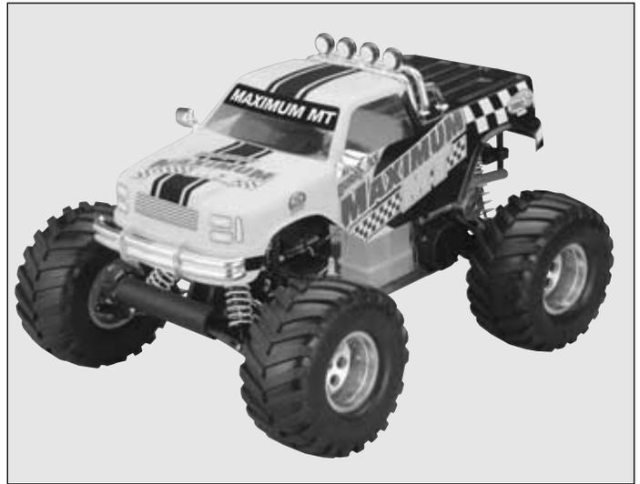
❑ 7. Mount the body on the body posts and secure the body to the truck with (4) body clips.
