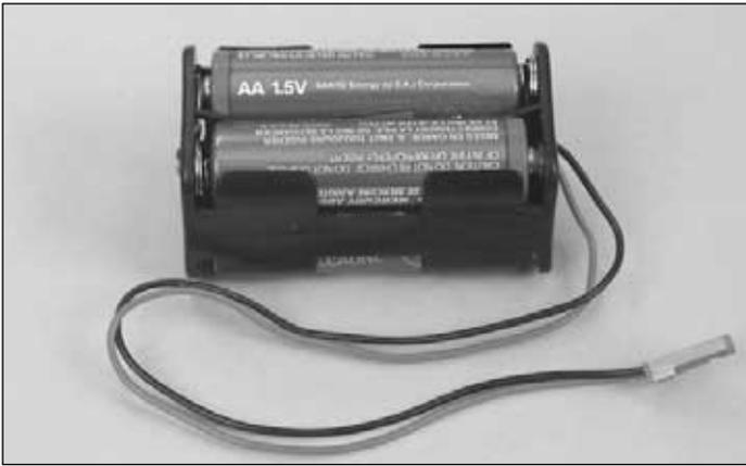
❑ 6. Remove the receiver battery holder from the radio box. Install (4) "AA" (included) into the battery holder in the configuration molded into the battery holder.
