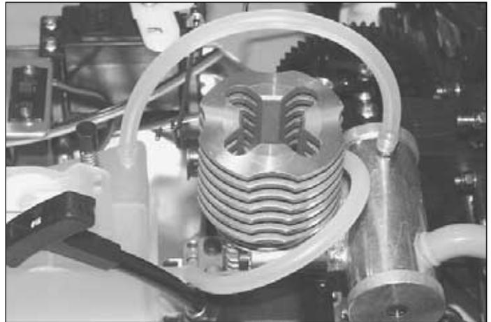
3. Cut the fuel line in half. Route one of the lines from the nipple on the top of the muffler to the top of the fuel tank. Route the other fuel line from the nipple on the carburetor to the bottom of the fuel tank. Ensure that the fuel line is not kinked anywhere along the line. You may have to shorten the line to eliminate kinks.
