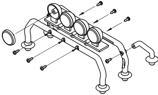
12. Assemble the rollbar as shown using ten 2.6 x 6mm self-tapping screws.
