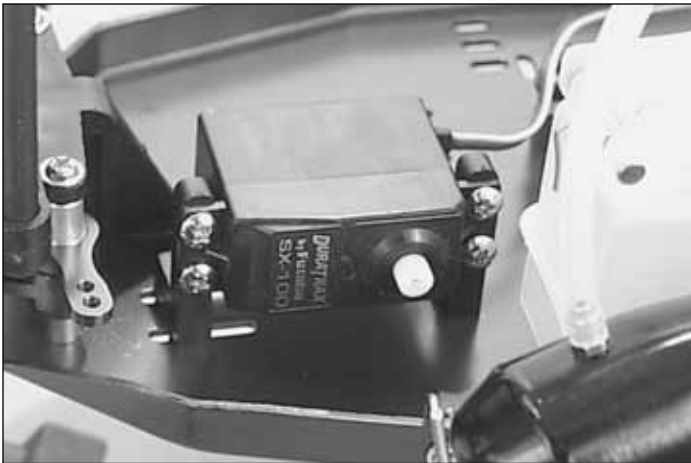
3. Attach the steering servo assembly to the chassis with (4) 3 x 8mm self-tapping screws in the holes provided as shown above.
