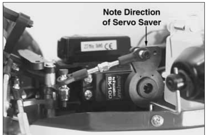
7. Place the servo saver onto the steering servo as shown.
