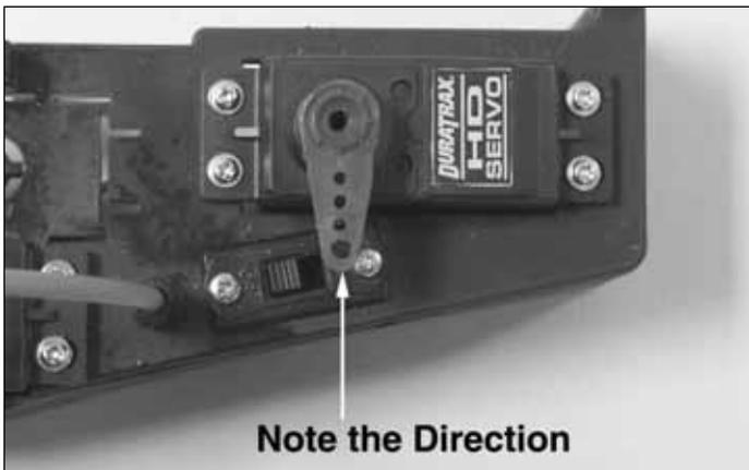
□ 12. Install the servo horn onto the steering servo, **note the direction of the servo horn**. Secure the horn to the servo with the screw included with the radio system.
