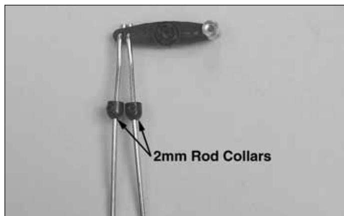
❑ 32. Install the set screw into two of the rod collars. Place one rod collar onto both of the pre-bent linkage rods. **Note: Do not tighten the set screws all the way down yet, the linkage will be adjusted later.**
