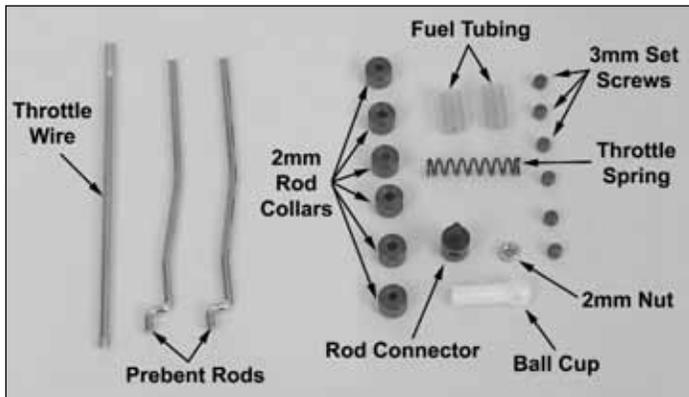
❑ 28. From the linkage bag remove the two remaining pre-bent linkage rods with z-bends at one end, the straight throttle wire, (6) 2mm rod collars, (6) 3mm set screws, (1) throttle linkage spring, (1) rod connector, (1) 2mm nut and (1) plastic ball cup. Also cut (2) 1/4" pieces of fuel tubing from the fuel tubing included with the kit.
