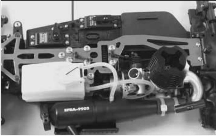
❑ 22. Re-install the radio box back onto the chassis. Use the (8) 3x15mm flathead self tapping screws that you removed earlier to secure the radio box back onto the chassis. Refer to the picture in step 2 on page 6.
