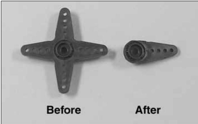
□ 11. Remove three of the arms off the steering servo horn as shown.
