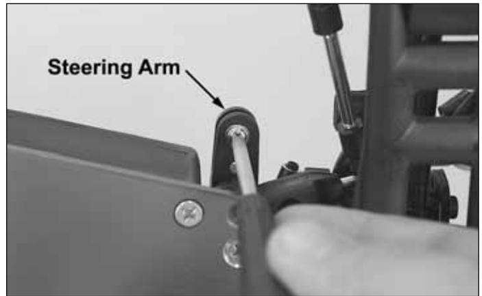
❑ 26. Loosen the screw in the bottom of the steering arm on the servo saver enough for the linkage rod to slide through the metal rod connector.
