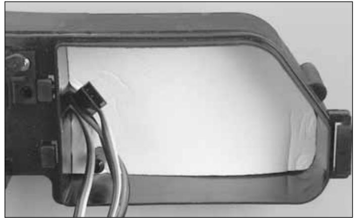
□ 13. Route the wires and connectors for the switch and two servos through the hole in the radio box. Cut a piece of foam the size of the radio box and place it in the bottom for all of the equipment to set on. Make sure that all of the wires coming into the radio box are on top of the foam. This is to help prevent vibration damage to the receiver.
