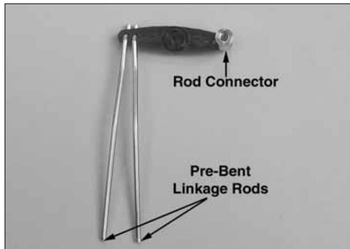
❑ 31. Install the two linkage rods with the z-bends at one end of them into the two enlarged holes at the opposite end from the rod connector.
