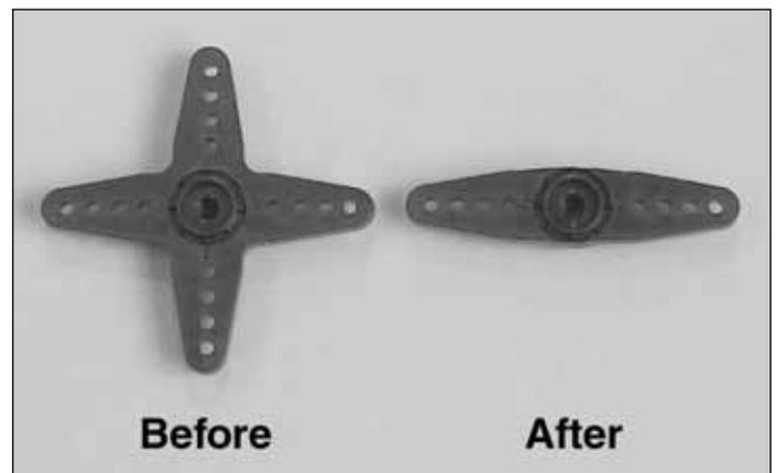
❑ 9. Cut two of the arms off the throttle servo horn by scoring both sides of the arm with a hobby knife and snapping off the arms with pliers.
