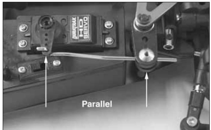
❑ 27. Remove the screw from the steering servo horn. Slide the steering linkage rod through the hole in the linkage rod connector in the steering arm. Place the servo horn back onto the servo. When placing the horn onto the servo, the horn and the steering arm should be parallel as shown in the photo. **Note: Do not screw the servo horn down yet, the servos will need to be centered after assembly is completed.**
