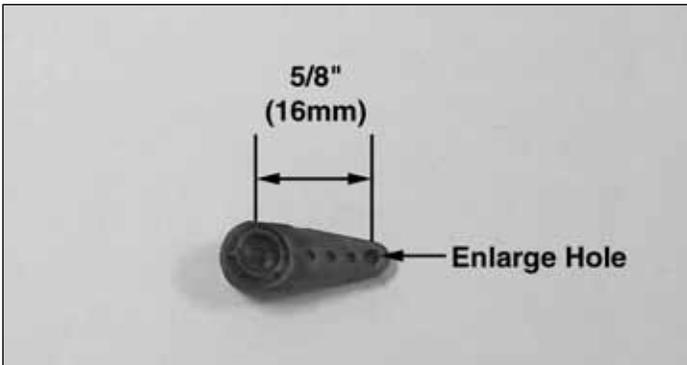
❑ 24. Remove the servo horn from steering servo. Using a 5/64" (2mm) drill bit or hobby knife, enlarge the hole 5/8" (16mm) away from the center of the horn.
