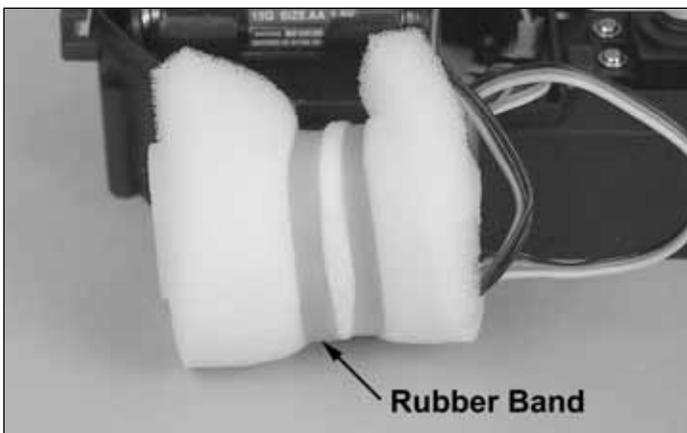
❑ 18. Cut a 2" x 7" (50 x 175mm) piece of the included foam and wrap it around the receiver. If desired, you can wrap a small rubber band (not included) around the outside of the foam to secure it in place for added security.
