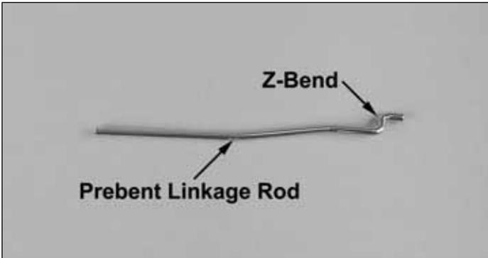
❑ 23. Remove one of the three pre-bent linkage rods with a z-bend at the end of it from the linkage bag. **Note all of the pre-bent rods are the same.**
