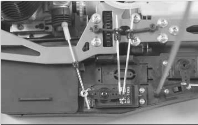
❑ 34. Screw the plastic ball cup onto the throttle linkage wire. Install one rod collar onto the linkage rod, then slide on the throttle linkage spring. Insert the throttle linkage through the rod connector as shown. **Note: Do not tighten the set screw in the rod collar down, adjustments will be made later.**
