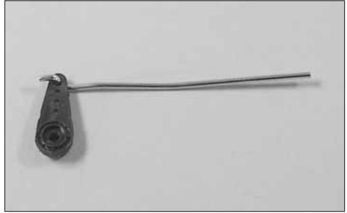
❑ 25. Install the z-bend end of the linkage rod into the servo horn from the bottom as shown.
