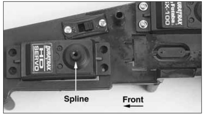
❑ 7. Place the high torque steering servo into the radio tray. **Note the direction of the servo spline when installing.** Run the servo lead through the hole in the side of the radio box.
