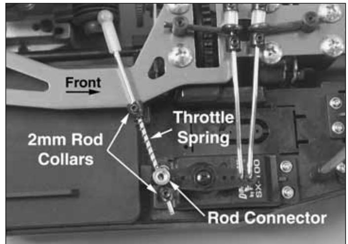
❑ 47. With the throttle servo still in neutral, push the throttle rod so that the carb closes. Move the rod collar against the rod connector and tighten the set screw. Move the other rod collar so that the throttle spring is *slightly* compressed and tighten the set screw.
