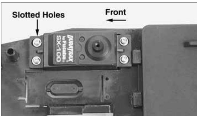
❑ 6. Mount the servo to the radio tray using four mounting screws included with the radio system. Use one of the servo mounting blocks that you cut out of the radio tray in step 4 and place it against the under side of the radio tray under the slotted holes. The screws should go through the servo, the radio tray and thread into the servo mounting block. **Note: Make sure to use the servo mounting block on the end with the slotted mounting holes.**
