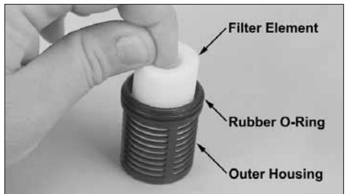
❑ 40. Assemble the air filter. Slide the large rubber O-ring around the threads of the outer housing. The O-ring will help seal the air filter housing together.
