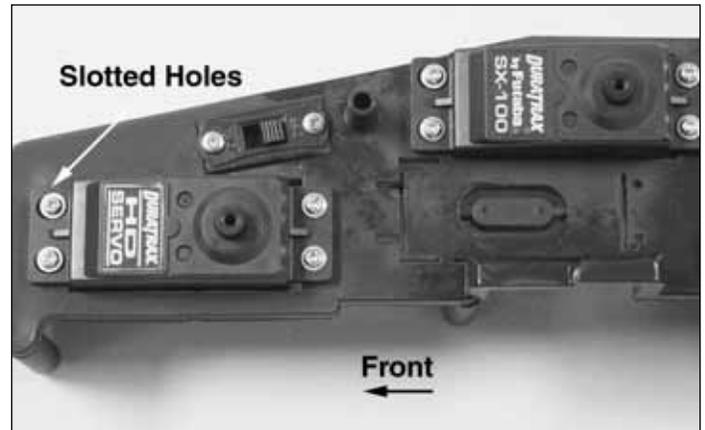
❑ 8. Mount the servo to the radio tray using four mounting screws included with the radio system. Use the other mounting block that you cut out of the radio tray in step 4 and place it against the under side of the radio tray under the slotted holes. The screws should go through the servo, the radio tray and into the servo mounting block. **Note: Make sure to use the mounting block on the end with the slotted mounting holes.**
