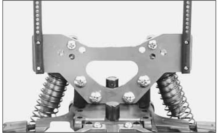
❑ 11. Remove the lower screw from each of the body posts so that the posts can be placed upright. Re-install the screw through the shock tower into the body post as shown.
