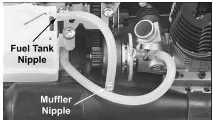
❑ 39. Install one end of the 4" (100mm) piece of fuel tubing onto the nipple next to the fuel tank lid and the other end on the nipple on the muffer.
