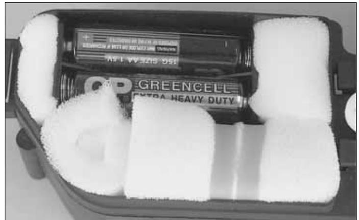
❑ 20. Cut the left over foam into small pieces and place them around the receiver and battery to help secure them into place. Then slide the radio box cover back onto the radio box.
