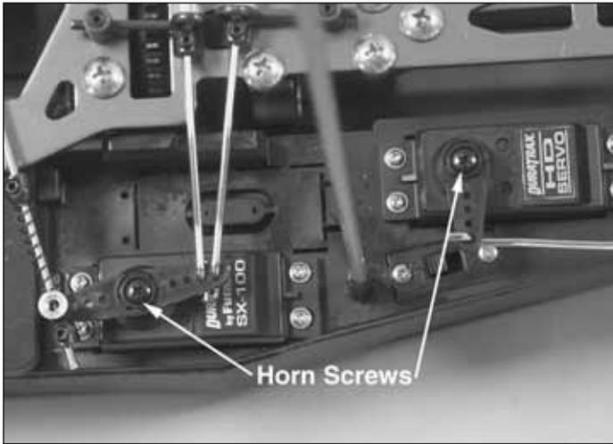
❑ 48. With the transmitter and receiver still on, remove the steering servo horn. While the front wheels are positioned straight, re-install the steering servo horn, so that the wheels remain as straight as possible. The fronts of the wheels may be slightly inward (that's O.K., this is called "toe-in", see page 17.)
