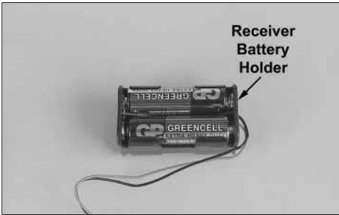
❑ 16. Install 4 “AA” batteries (not included) into the receiver battery holder in the configuration molded into the battery holder included with the radio system.
