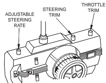
**6.** Make sure the front wheels of the Nitro Evader move left and right correctly when the transmitter wheel is turned.
