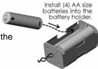
Install (4) AA size batteries into the battery holder.
