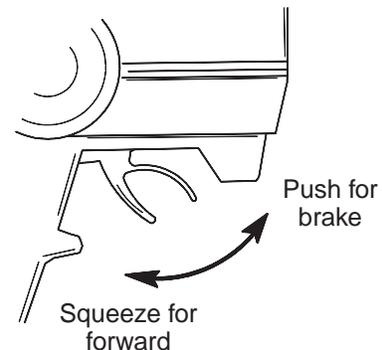
**5.** Make sure the throttle opens all the way when the throttle is applied on the transmitter. Make sure the brakes work adequately when the trigger is pushed forward.
