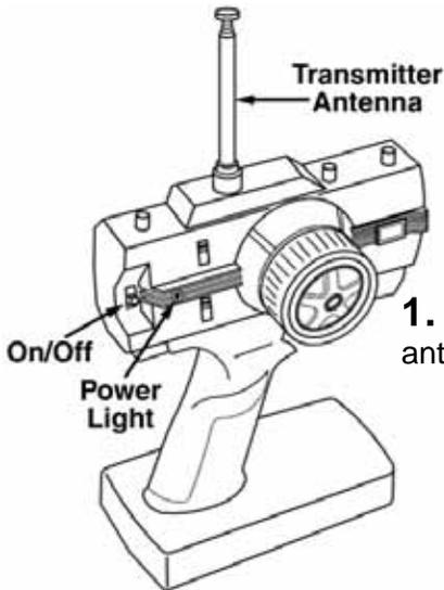
**1.** Install the transmitter antenna into the transmitter.
