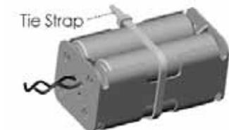
**5.** Use a tie strap to secure the batteries in the holder.
