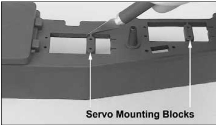
❑ 4. Use a hobby knife or diagonal cutters to remove the servo mounting blocks from the radio tray. Make sure all of the flashing is removed from inside the servo compartment to assure a proper servo fit. **Save the servo mounting blocks.**
