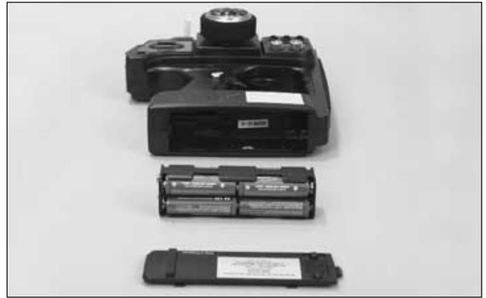
❑ 10. Slide open the battery door on the bottom of the transmitter and remove the transmitter battery holder. Place 8 “AA” batteries (included) into the holder in the configuration molded into the plastic on the battery holder. Re-install the transmitter battery holder into the transmitter and re-install the battery door.
