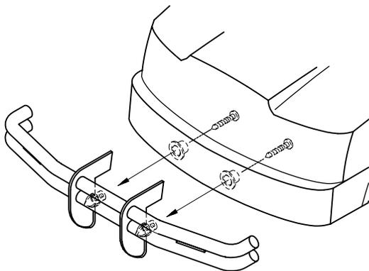
□ 15. Drill two 1/4" (6mm) holes in front of body using the molded-in dimples as guides. Install the front brush guard as shown with two 2.6 x 6mm self-tapping screws and the collars included.
