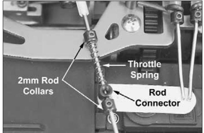
❑ 47. Tighten the rod collar that retains the throttle spring so that the spring cannot move back and forth but not so much that the spring is tight. The rod collar at the other end of the throttle linkage should be tightened against the rod connector as shown.
