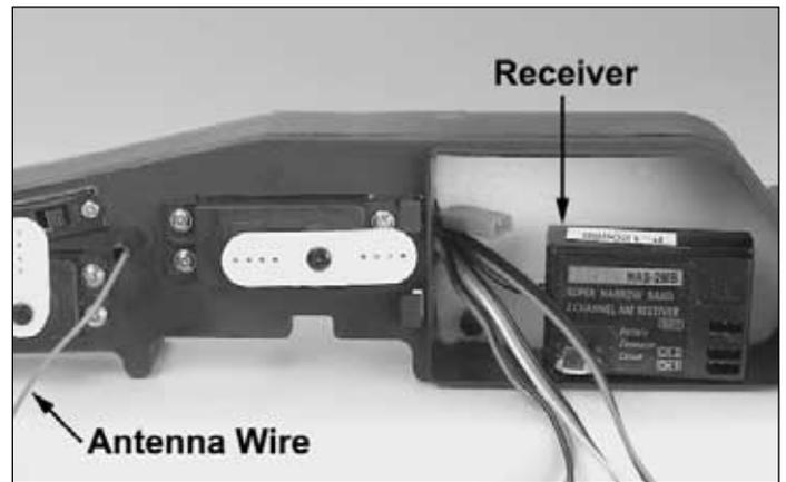
❑ 14. Install the receiver into the radio box and route the antenna wire through the same hole the servo leads come in. Run the antenna wire up through the antenna mount hole.
