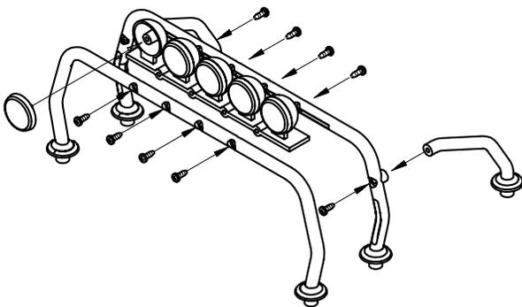
❑ 51. Assemble the rollbar as shown using ten 2.6 x 6mm self-tapping screws.
