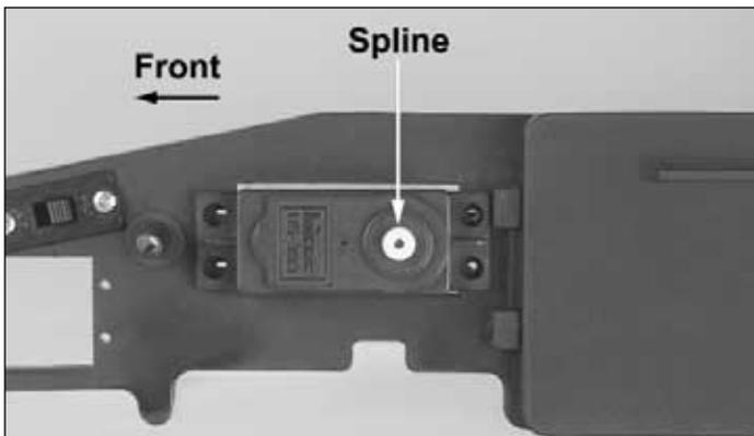
❑ 5. Place the standard throttle servo into the radio tray. **Note: Notice the direction of the servo spline when installing.** Run the servo lead through the hole in the side of the radio box.
