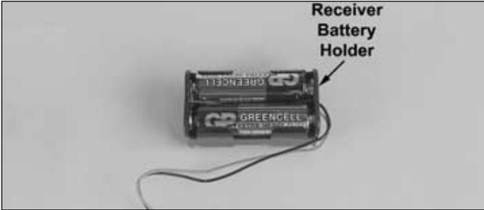
❑ 7. Remove the receiver battery holder from the radio box. Install (4) “AA” batteries (included) into the battery holder in the configuration molded into the battery holder.
