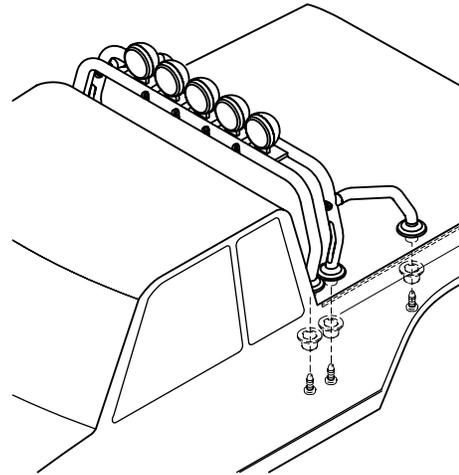
❑ 52. Drill six 1/4" (6mm) holes in the body using the molded-in dimples as guides. Install the rollbar onto body as shown using six 2.6 x 6mm self-tapping screws and the included collars.
