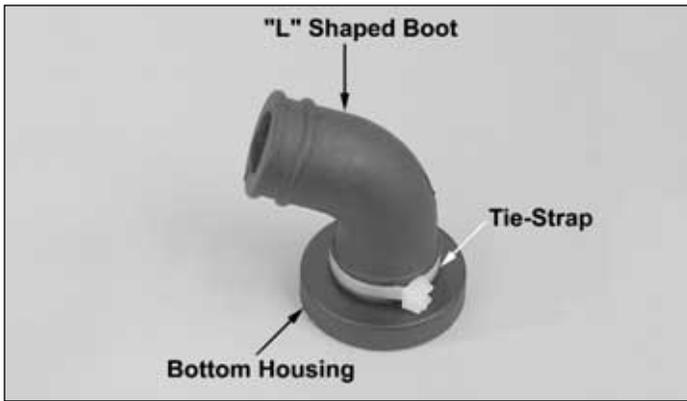
❑ 42. Press the "L" shaped boot onto the bottom housing of the air filter. Using one of the included tie-straps, secure the boot tightly onto the bottom housing. Cut the excess portion of the tie-strap to avoid interference.
