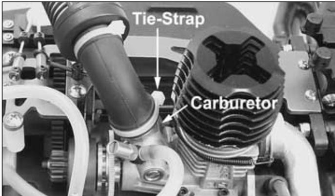
❑ 44. Place the air filter onto the carburetor. Using the remaining included tie-strap, tightly secure the air filter to the carburetor. Cut the excess portion of the tie-strap off to avoid interference.
