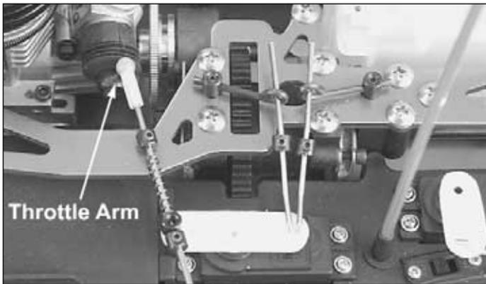
❑ 35. Snap the ball cup onto the throttle arm. Install a second rod collar onto the throttle linkage so that it fits against the rod connector. **Note: Do not tighten the set screw in the rod collar, the linkage will be adjusted later.**
