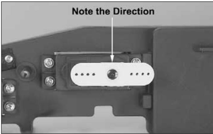
❑ 10. Install the servo horn onto the throttle servo, **note the direction of the servo horn**. Secure the horn to the servo with the screw included with the radio system.
