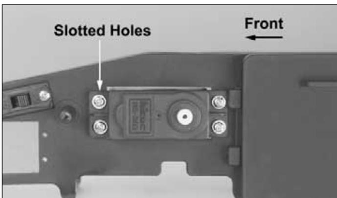
❑ 6. Mount the servo to the radio tray using four mounting screws included with the radio system. Use one of the servo mounting blocks that you cut out of the radio tray in step 4 and place it against the under side of the radio tray under the slotted holes. The screws should go through the servo, the radio tray and into the servo mounting block. **Note: Make sure to use the servo mounting block on the end with the slotted mounting holes.**
