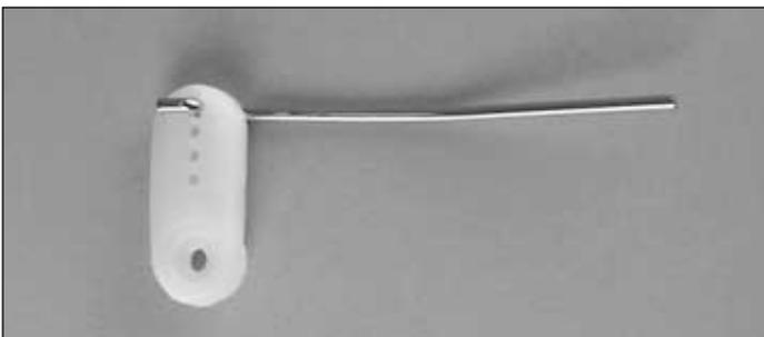
❑ 25. Install the z-bend end of the linkage rod into the servo horn from the bottom as shown.
