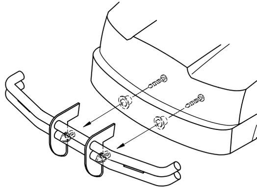
❑ 53. Drill two 1/4" (6mm) holes in front of body using the molded-in dimples as guides. Install the front brush guard as shown with two 2.6 x 6mm self-tapping screws and the collars included.
