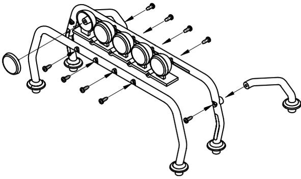
□ 13. Assemble the rollbar as shown using ten 2.6 x 6mm self-tapping screws.
