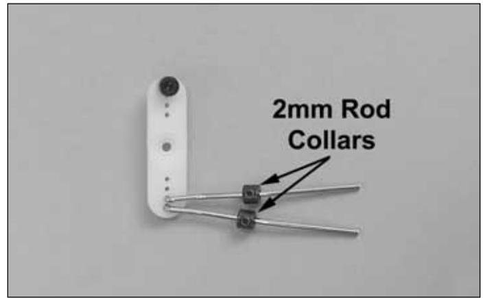
❑ 32. Install the set screw into two of the rod collars. Place one rod collar onto both of the prebent linkage rods. **Note: Do not tighten the set screws all the way down yet, the linkage will be adjusted later.**
