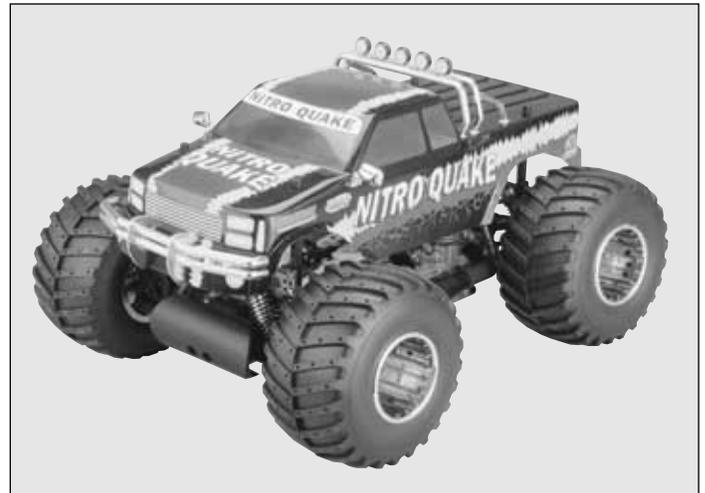
□ 17. Remove the body clips from the parts bag. Place the body onto the body mounts. On each body mount place a body clip.
