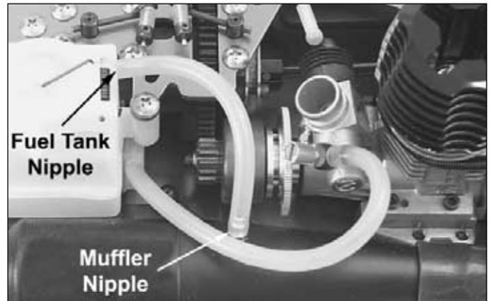
❑ 39. Install one end of the 4" (100mm) piece of fuel tubing onto the nipple next to the fuel tank lid and the other end on the nipple on the muffler.
