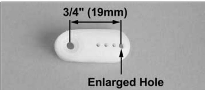
❑ 24. Remove the servo horn from steering servo. Enlarge the hole 3/4" (19mm) away from the center of the horn with a 5/64" (2mm) drill or a hobby knife.
