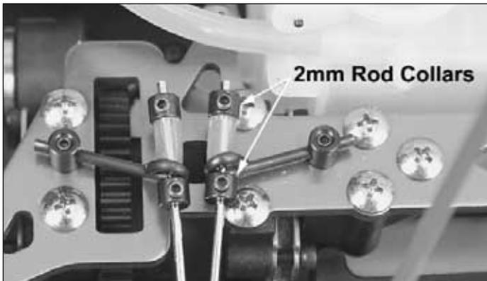
❑ 46. Slide the rod collars and fuel tubing that engage the brakes so that when the car is at an idle the brakes
