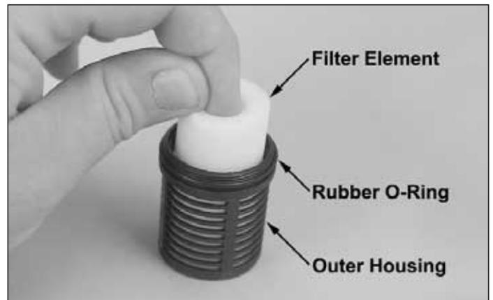
❑ 40. Assemble the air filter. Slide the large rubber O-ring around the threads of the outer housing. The O-ring will help seal the air filter housing together.
