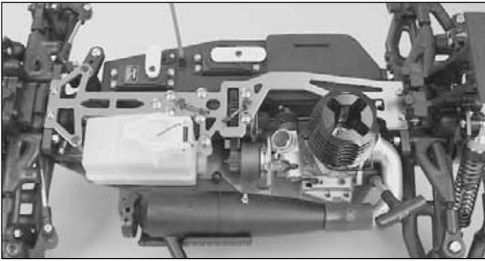
❑ 22. Re-install the radio box back onto the chassis. Use the (8) 3x15mm flathead self tapping screws that you removed earlier to secure the radio box back onto the chassis. Refer to the picture in step 2 on page 6.
