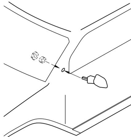
❑ 54. Drill one 1/8" (3mm) hole in each side of the body using the molded-in dimple as a guide. Install the mirrors as shown with the collars and nuts provided.
