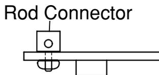
❑ 30. Install the rod connector into the top of the horn at the end with the single enlarged hole. Apply a small amount of thread locking compound onto the threads of the rod connector, then thread on the 2mm nut. Do not overtighten the nut, the rod connector must be able to swivel freely.
