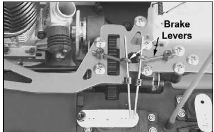
❑ 33. Re-install the servo horn onto the servo. Slide the brake linkage rods through the brake levers as shown.
