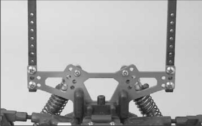
❑ 49. Remove the lower screw from each of the body posts so that the posts can be placed upright. Re-install the screw through the shock tower into the body post as shown. The height of the body can be adjusted by raising or lowering the posts on the shock tower.
