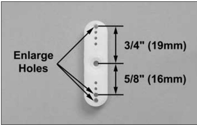
❑ 29. Remove the servo horn from the throttle servo. Enlarge the two farthest holes at one end of the horn and the farthest hole on the other end with a 5/64" (2mm) drill or a hobby knife.
