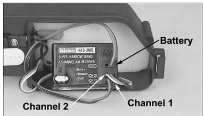
❑ 15. Plug the steering servo, throttle servo and switch into the receiver. See your radio instructions to determine which channel is steering and which is throttle. The switch plugs into the battery socket.
