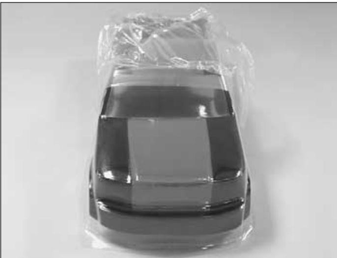
❑ 50. Remove the plastic from the outside of the body. Apply the decals to the body if desired.
