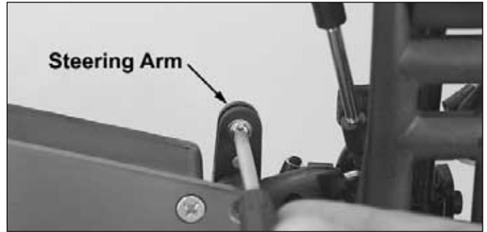
❑ 26. Loosen the screw in the bottom of the steering arm on the servo saver enough for the linkage rod to slide through the metal rod connector.
