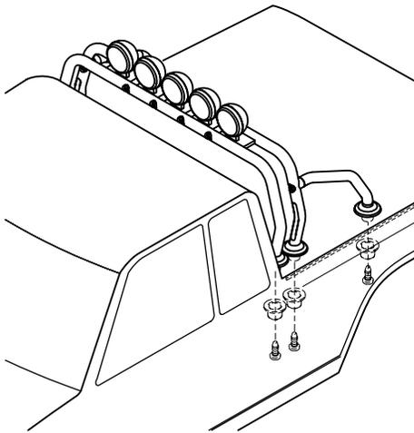
□ 14. Drill six 1/4" (6mm) holes in the body using the molded-in dimples as guides. Install the rollbar onto body as shown using six 2.6 x 6mm self-tapping screws and the included collars.
