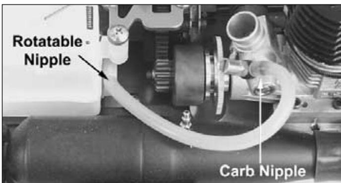
❑ 38. Install one end of the 6" (150mm) piece of fuel tubing onto the rotatable nipple on the rear of the fuel tank and the other end onto the nipple on the carburetor.
