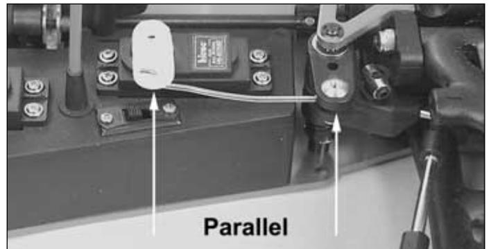
❑ 27. Remove the screw from the steering servo horn. Slide the steering linkage rod through the hole in the linkage rod connector in the steering arm. Place the servo horn back onto the servo. When placing the horn onto the servo, the horn and the steering arm should be parallel as shown in the photo. **Note: Do not screw the servo horn down yet, the servos will need to be centered after assembly is completed.**
