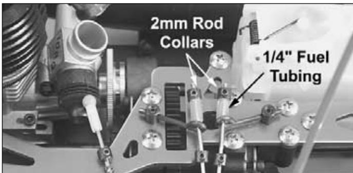
❑ 36. Slide a 1/4" piece of fuel tubing over each of the brake linkage rods. Then install a rod collar onto each of the two rods. **Note: Do not tighten the set screw in the rod collars, the linkage will be adjusted later.**
