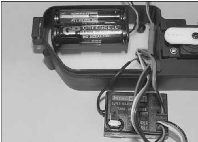
❑ 17. Install the receiver battery into the radio box. Note the placement of the receiver battery in the box. Connect the receiver battery to the remaining end of the on/off switch.
