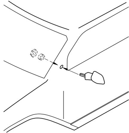
□ 16. Drill one 1/8" (3mm) hole in each side of the body using the molded-in dimple as a guide. Install the mirrors as shown with the collars and nuts provided.
