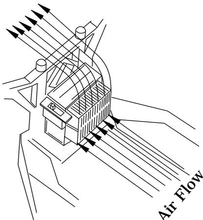
Mount the speed control to obtain maximum parallel airflow THROUGH the heat sink. For off-road cars, or cars with a metal or graphite chassis, mount the ESC on the chassis, and the receiver and antenna on the rear shock tower to reduce radio interference.
