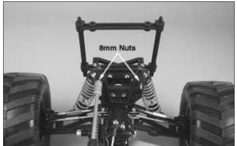
26) Reattach the shocks to the shock tower by re-installing the 8mm nuts.
