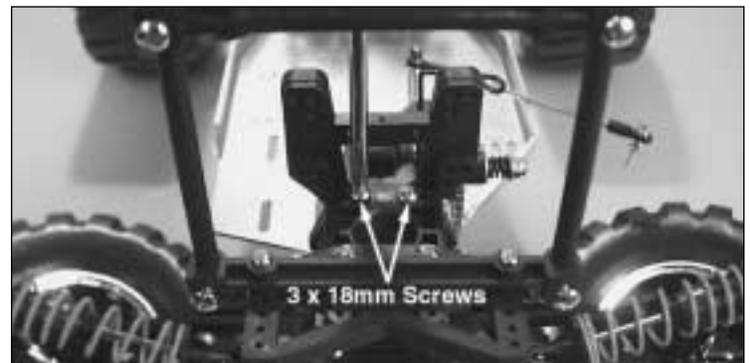
11) Remove the body mount assembly by removing the two 3 x 18mm screws.
