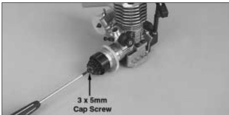
7) Remove the 5 x 10mm flanged bearing from the old clutch bell and install it into the end of the new clutch bell and slide it onto the pilot shaft. Apply a small amount of thread lock to the 3 x 6mm cap screw and insert into the end of the pilot shaft to secure the clutch bell to the engine.
