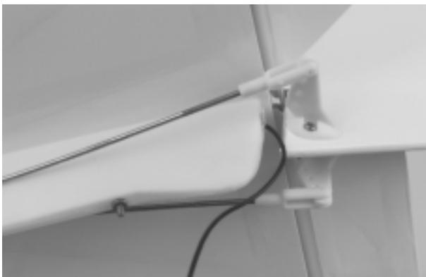
**Step 3.** Make sure the rudder and elevator servo arms are centered, and attach the metal pushrods to the respective servo arms. The control linkage length can be adjusted by threading the clevis at the control horn in or out.
