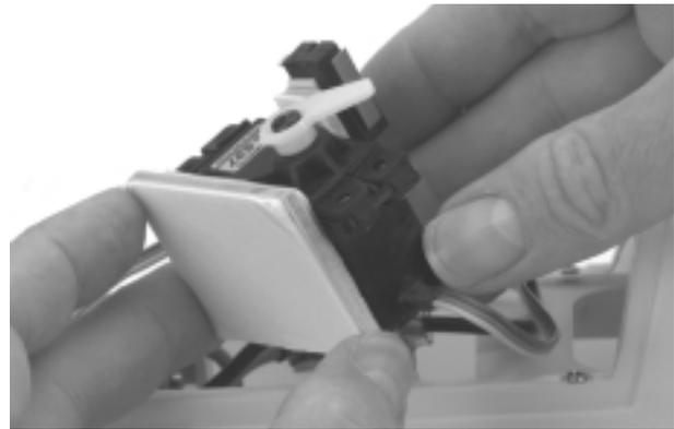
**Step 13.** Place the plywood plate with the micro switch/servo into the area of the fuselage aft of the motor near the arming switch position and attach with double-sided servo tape.
