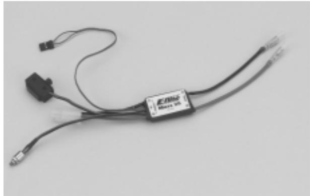
**Step 10.** The micro-switch is used to turn the motor on and off in flight. Use double-sided servo tape to attach the micro-switch to the side of the servo as shown below.
