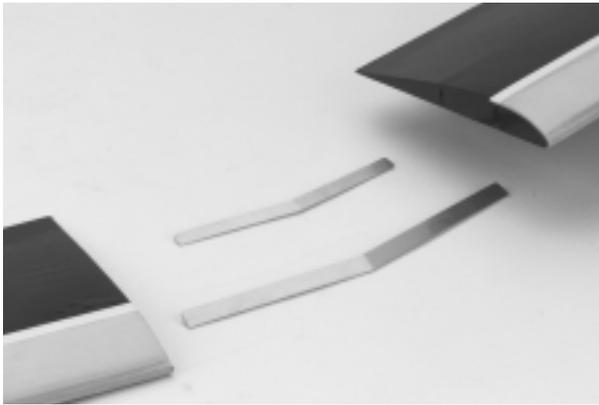
**Step 2.** Trial fit the two wing joiners (dihedral braces) into one of the wing halves. They should insert smoothly. Now slide the other wing half onto the wing joiners until the wing halves meet.
