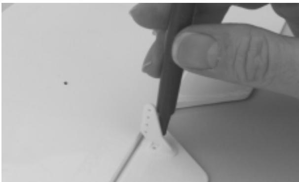
**Step 3.** Mark the post where the horn will be placed using a felt-tipped marker and drill the marked locations using a 1/16" drill bit.
