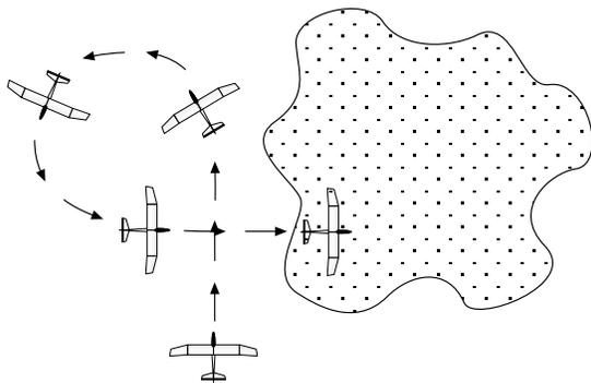
The second method is to make a wide 180-degree turn back into the thermal.
