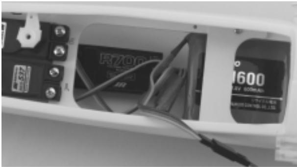
**Step 7.** The receiver antenna will be run from the opening in the fuselage area out to the fuselage tail.
