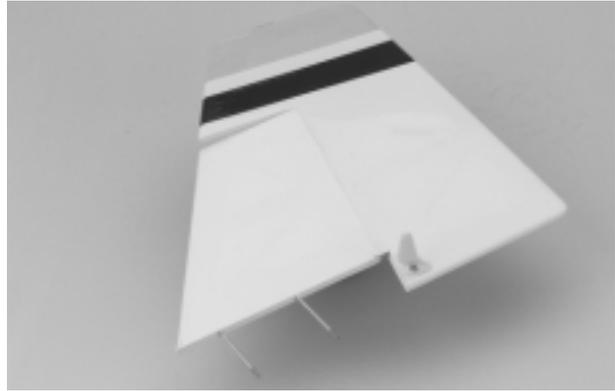
**Step 4.** Mount the vertical fin and rudder to the horizontal stabilizer and elevator by sliding the two metal rods through the holes in the horizontal stabilizer. Then push the rods through the fuselage and lock them in place using an adjustable wrench the two 2 mm nuts. Use blue Locktite on the threads to secure the nuts in place.
