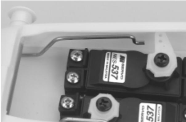
**Step 2.** Check to see that the clevis for the elevator and rudder are attached and a clevis keeper (piece of fuel tubing) is installed.
