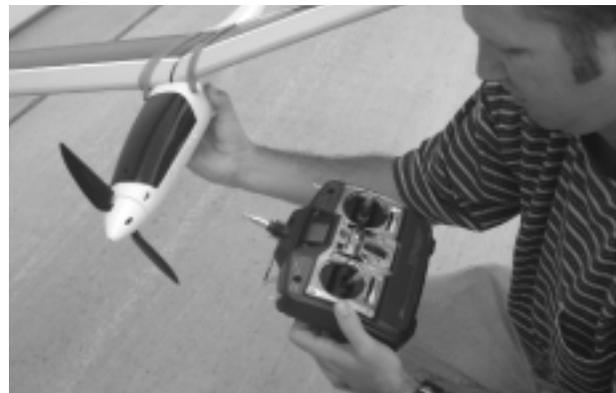
**Step 5.** Make any necessary adjustments to control linkages, or servo arm position to micro-switch so that the controls move freely without any servo binding and that the motor turns on and off. Also check to make sure the "Arming" switch functions properly by having the system on and running, and then turning off the arming switch. The motor should stop.
