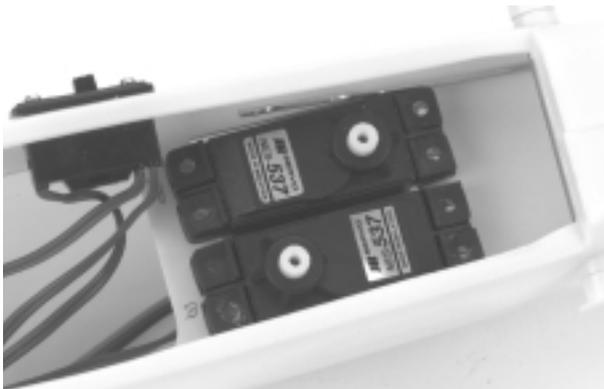
**Step 3.** Using a Phillips screwdriver, screw the eight screws to secure the servos.
