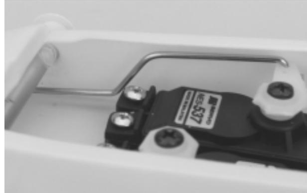
**Step 4.** With the rudder and elevator pushrods attached, and the micro switch/servo installed, check the function of the controls by turning on the transmitter, then the receiver.
