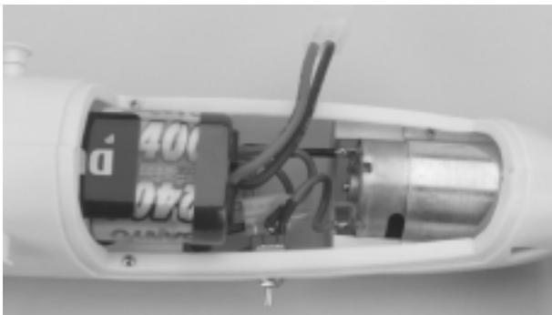
**Step 9.** A micro On/Off switch and a single-pole/double-throw switch are installed in the sides of the fuselage near the motor and the radio compartment. The micro switch is to power the receiver and the single pole/double throw switch is an "arming switch." The arming switch prevents unwanted power from being applied to the motor and prevents accidental startup. Remember the propeller has sharp edges and can cause injury if you stick your hand or fingers into it when it is operating.
