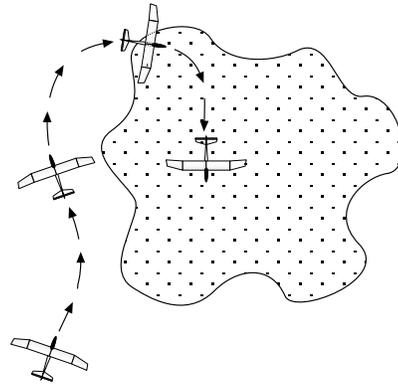
Once in the thermal, you will need to try to stay in the center of the lift. Slow down by increasing the up elevator "trim" until the sailplane is just above a stall (minimum sink speed). Make easy banking turns to find the area of highest lift (thermal core). When you have found the core of lift, tighten the turns to stay within the core of highest lift.
