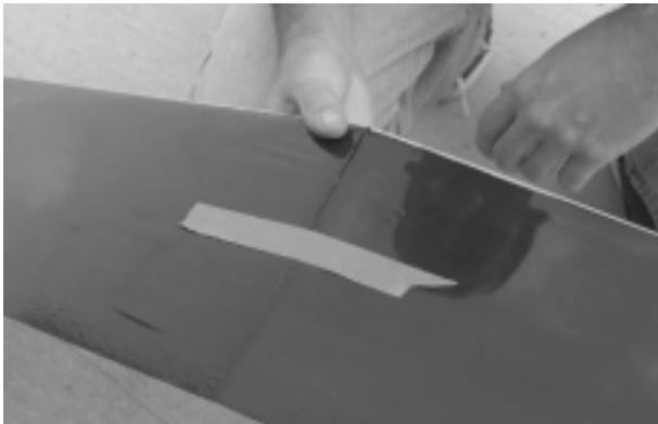
**Step 3.** Mark the location of the CG on the bottom of the wing either side of the fuselage.
