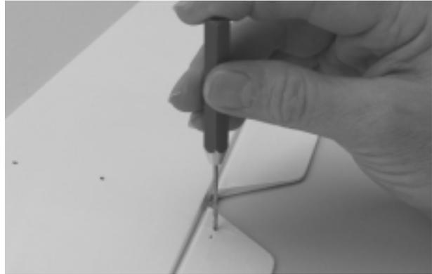
**Step 4.** Mount the rudder control horn to the vertical fin/rudder using the two screws and nuts provided. Mount the control horn on the left side of the rudder using the same method as above.
