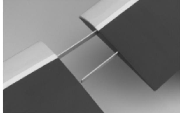
**Step 3.** Tape the wing halves together using scotch tape. This allows for easy breakdown of the wing for transportation.
