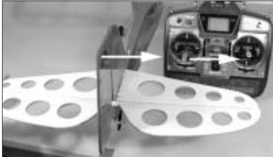
2. Check the movement of the elevator with the radio system. Moving the elevator stick down will make the airplane elevator move up.
