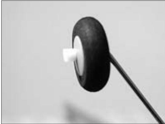
**Note:** Do not get CA between the wheel and landing gear.
