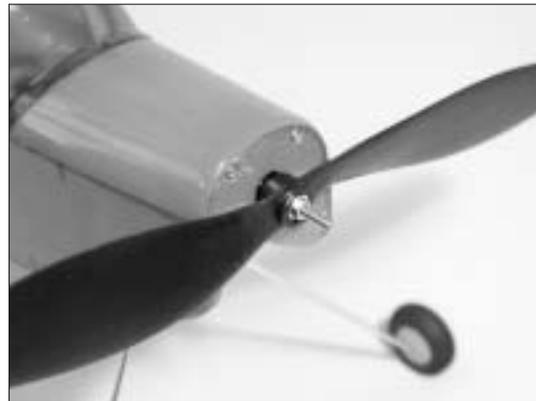
**Note:** The text on the propeller faces the front of the airplane.
