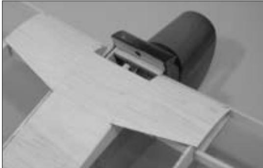
2. Secure the wing to the fuselage using a 4-40 x 1/2" socket head bolt and a #4 flat washer.
