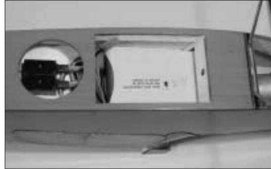
2. Place the battery hatch onto the fuselage. Use a 3/32" hex wrench to install the 4-40 x 1/2" screw and #4 washer.
