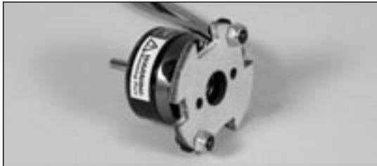
2. Slide the motor into position in the fuselage. Glue the plywood mount to the fuselage using foam-safe CA. Trim the fuselage as necessary to clear the motor and wiring to the motor.
