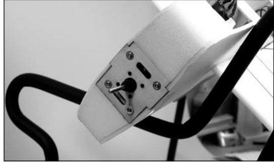
**Hint:** You may want to plug in the speed control before installing the gearbox.
