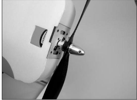
**Note:** If using a direct drive Outrunner motor, a smaller prop is needed. Use 11 x 4.7 for the Park 400 Outrunner, 920 Kv or use a 10 x 4.7 for the Park 370 Outrunner, 1080 Kv.
