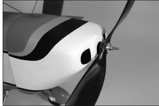
**Note:** It is very important that you check to be sure the propeller is balanced before installing onto the shaft. An unbalanced propeller may strip the gear. When installing the propeller, please do not over-tighten the 3mm locknut. The use of the locknut will prevent the propeller from falling off in flight.
