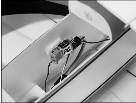
**Note:** Do not cut the receiver antenna. Changing the length of the antenna will seriously reduce the range of your radio system.
