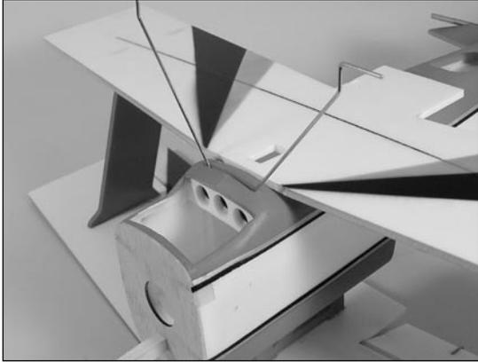
**Note:** If the landing gear is loose and you choose to permanently attach the gear, use foam compatible CA to glue the plywood landing gear retainer into the slot.
