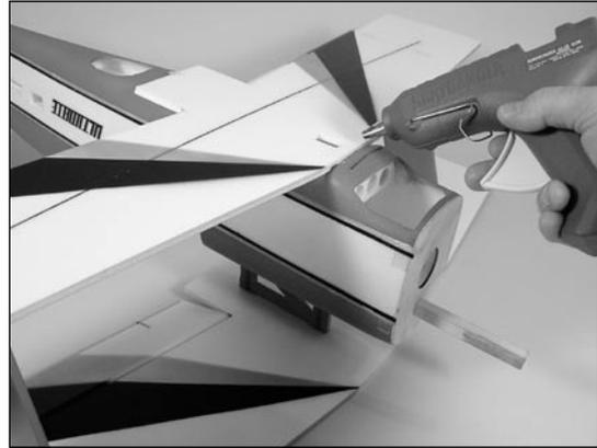
**Note:** The long brace (11 <sup>3</sup>/<sub>4</sub>" ) goes from the top near the cabane to the strut on the bottom wing.
