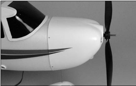
**Note:** If you have selected the outrunner motor option, install the propeller adapter onto the motor shaft.
