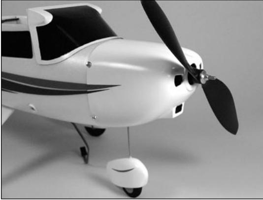
**Note:** Simply tighten the adapter when using the outrunner and associated propeller mounting hardware.
