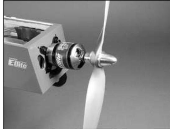
**Note:** It is very important that you check to be sure the propeller is balanced before installing onto the shaft. An unbalanced propeller will cause performance issues.
