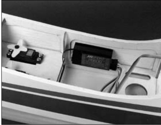
**Note:** Do not cut the antenna wire, as this will reduce the range of your radio system.
