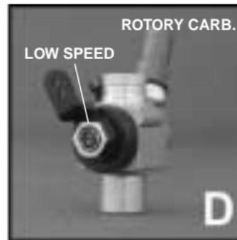
**IMPORTANT:** Carburetors are very sensitive to minor adjustments. Any adjustments should be made in increments of 1/16th to 1/8th of-a-turn, at a time. New carburetors should be set to the following guidelines and are not considered pre-set from the factory.
