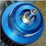
5. Slide the gold spring over the crankshaft and into the plate.
