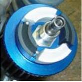
4. Place the clutch plate over the pads. Check to make sure the pads seat properly in the groove of the plate.
