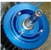
2. Apply a drop of medium strength thread lock compound to the flywheel nut and thread onto the crankshaft, securing the flywheel in place.
