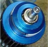
6. Apply a drop of medium strength thread lock compound to the spring nut and install onto the threads of the flywheel nut about ¼ turn or just enough to keep the spring nut from falling off. Before installing clutch bell, see below for final adjustment and tuning tips.
