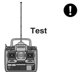
**! Check that the transmitter (Tx) antenna is not loose.**
