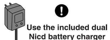
**Do not short the nicd battery connector terminals.**
