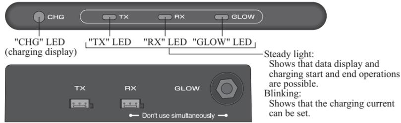
Connect the charger to the output connector matched to the type of battery to be charged. The corresponding LED in the "TX", "RX", and "GLOW" LEDs lights. The charging current setting screen is also automatically displayed.
