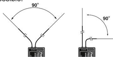
**4** If your model includes metal conductive items which may impact the receiver's ability to clearly receive the radio frequency signal, we suggest mounting the receiver so that the receiver antennas exit both sides of the model. This will allow the best radio frequency signal condition at any flying attitude.
