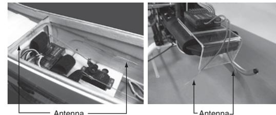
\* The main purpose of the photo demonstrates how the antenna should be placed. For actual installation the receiver must be wrapped with a sponge or placed with floating material to protect it from vibration.
