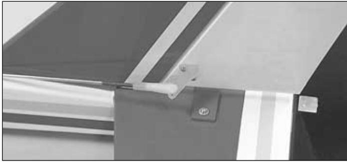
❑ 9. Install the rudder pushrod. Thread a **clevis** 14-turns onto the pushrod. Attach the clevis to the control horn. Bend the pushrod as necessary to allow for free movement.
