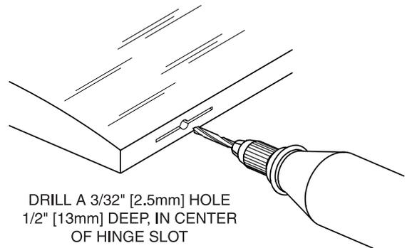
A. Drill a 3/32" [2.5mm] hole, 1/2" [13mm] deep, in the center of the hinge slot. If you use a Dremel® MultiPro™ for this task, it will result in a cleaner hole than if you use a slower speed drill. Drilling the hole will twist some of the wood fibers into the slot, making it difficult to insert the hinge, so you should reinsert the knife blade, working it back and forth a few times to clean out the slot.
