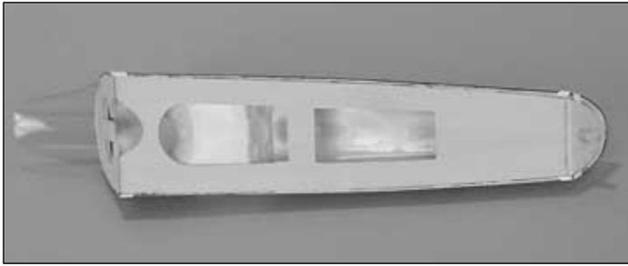
❑ 4. Trim the **cockpit**. Use CA to glue the cockpit to the canopy braces. Glue the dowel to the front canopy brace, allowing it to protrude 3/8" [9.5mm] out front.
