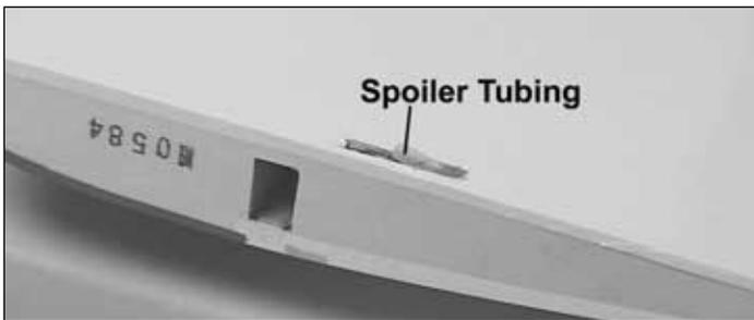
2. Pull the end of the spoiler tubing out of the wing just far enough to glue it in place using thick CA.
