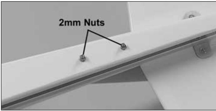
2. Open the holes on the top and bottom of the fuselage covering for the **fin** attachment. Attach the fin using two 2mm washers and two 2mm nuts. Use thread lock on the nuts to prevent loosening.
