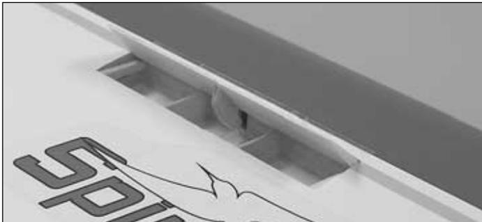
3. Cut the covering all around the edge of the **spoiler** and remove it from the wing panel.
