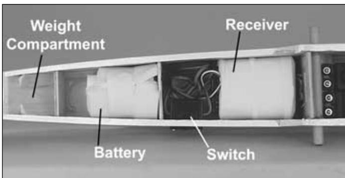
3. Install the receiver, battery and switch. Use foam to cushion the receiver and battery. Extend the antenna to the rear of the fuse.
