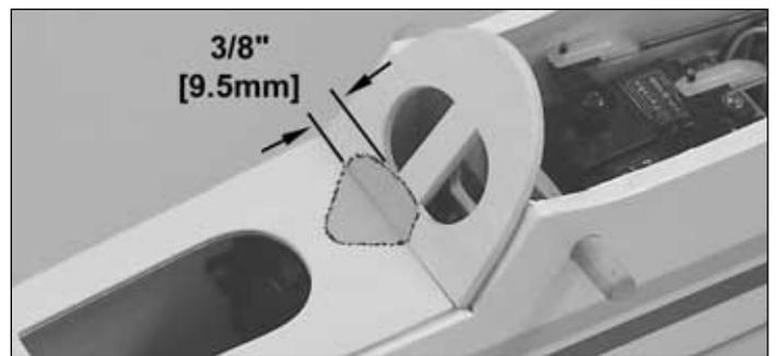
❑ 3. With the wax paper still in place, glue the **rear canopy brace** to the bottom canopy brace with CA. **Note:** If you are planning on using the optional spoilers, you must remove the shaded area to allow for servo movement.
