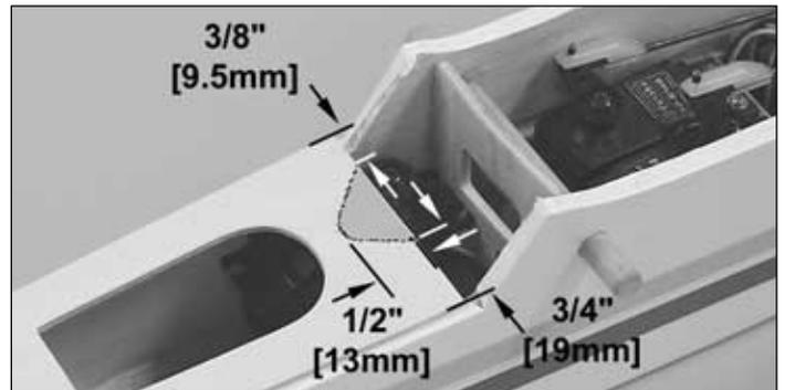
❑ 2. Place a piece of wax paper between the **bottom canopy brace** and fuselage. Glue the bottom canopy brace to the front canopy brace with CA. The wax paper will prevent the braces from accidentally being glued to the fuselage. **Note:** If you are planning on using the optional spoilers, you must remove the shaded area to allow for servo movement.
