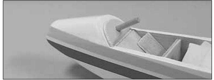
❑ 1. Place the small **hardwood dowel** into the **front canopy brace**. Remove the covering for the dowel in the front of the fuselage. Install the dowel into the hole.
