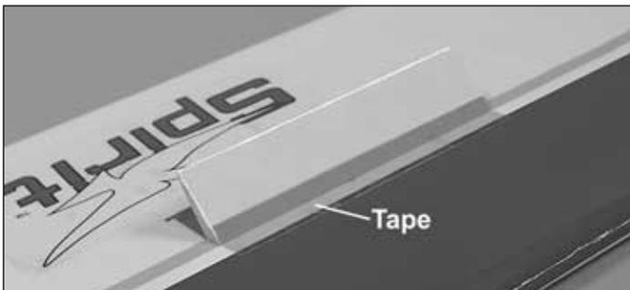
4. Tape the spoiler in position in the wing using a strip of cellophane or vinyl tape or a strip of covering. The tape should be flexible enough to allow the spoiler to close on its own. The tape should also be replaced occasionally as it will eventually rip.
