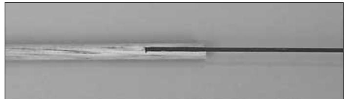
7. Insert one threaded piece of wire into each pushrod. Insert the remaining pieces of wire into the other end of each pushrod. Tack glue the wires in place with a couple drops of CA. Repeat the procedure to attach the non-threaded pushrod wires to the opposite end of the pushrod dowels.
