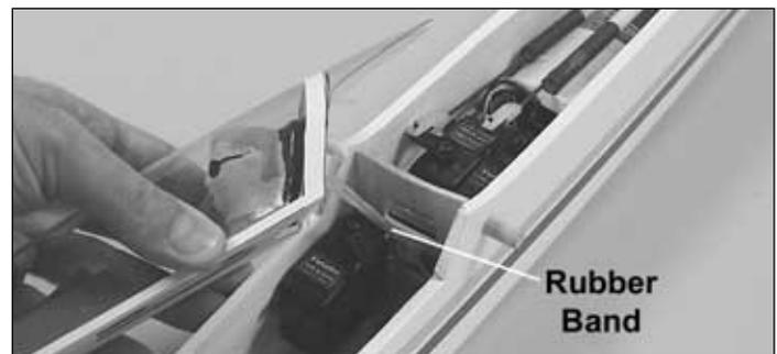
❑ 2. The canopy is held in place with a rubber band. Loop a medium size rubber band through the cut-out in the canopy back. Thread the rubber band through itself and then hook it on the little extension on the former. To remove the canopy, pick up on the back until the dowel is clear of the fuselage. To re-install the canopy just do the opposite.
