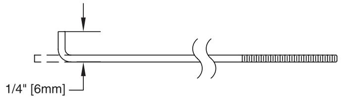
4. Make a 90° bend 1/4" [6mm] from the non-threaded end in each of the **pushrod wires** as shown in the sketch. Wipe off each wire using a paper towel dampened with rubbing alcohol to remove any oil. Make the same 90° bend in all four of the threaded and non-threaded pushrods.
