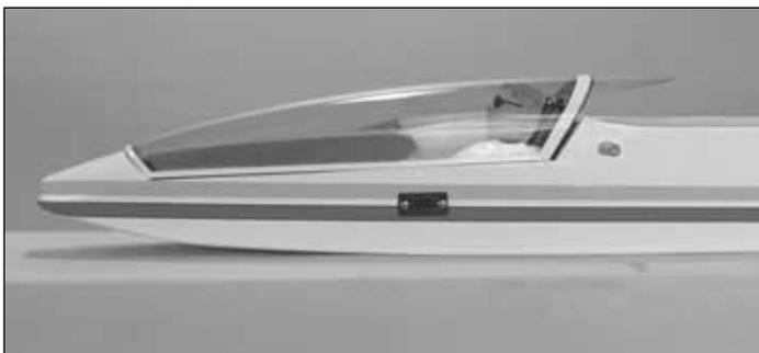
❑ 7. Test fit the canopy onto the fuselage. Trim the canopy flush with the base and the front but **do not trim the back yet!** Curved tip scissors works well for trimming the canopy. Temporarily mount the wing in place on the fuselage. **VERY CAREFULLY** trim the back of the canopy, **A LITTLE AT A TIME**, to fit over the wing. Take your time and use the outlines and the wing for guides.
