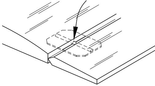
□ □ D. Add six drops of thin CA to the center of the hinges on both sides. Use a paper towel to absorb excess CA from the hinge gap before it cures. Do not use CA accelerator; allow the CA to cure slowly.
