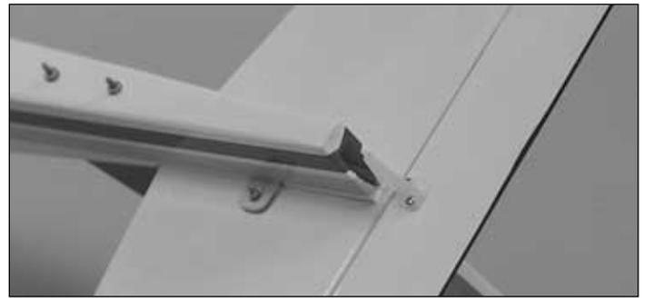
□ 7. Position the remaining control horn in line with the center of the fuselage on the bottom of the elevator. Attach the control horn to the elevator using two 2mm x 15mm screws.
