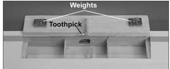
6. Thread one end of the line through the small hole in the spoiler horn and use a piece of a round toothpick to hold the line in the horn. Allow about 1/2" [13mm] to hang out the other side of the horn for fine adjustments. It may be necessary to drill out the spoiler control horn using a 3/32" [2.5mm] drill bit. Trim the shear web to allow the toothpick to pass through without interference.
