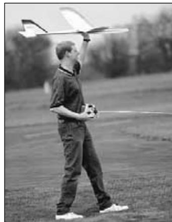
Turn on the transmitter first and then the receiver. Hold the SPIRIT ARF under the wing with the nose pointed slightly
