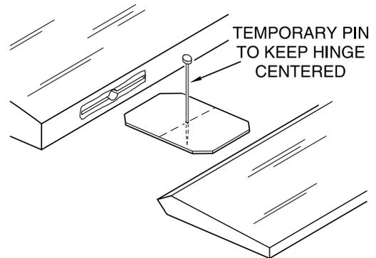
B. If the hinges don't remain centered, remove the rudder and insert a pin in the center of the hinges.
