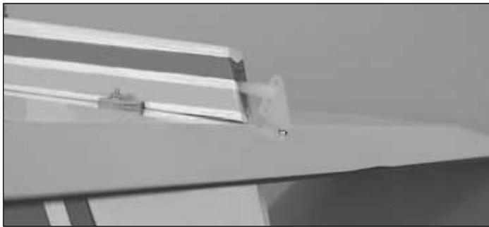
❑ 10. Install the elevator pushrod. Thread the clevis onto the pushrod. Attach the clevis to the control horn. Trim the opening at the rear of the fuselage as necessary to allow the pushrod to move freely.
