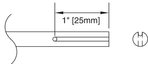
6. Drill a 5/64" [2mm] hole 1" [25mm] in from both ends of each pushrod. Cut a groove in the dowel from the hole to the end of the dowel.
