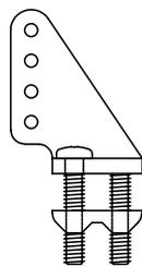
□ 6. Position one of the **nylon control horns** up 1/2" [13mm] up from the bottom of the rudder. Align the horn parallel to the bottom of the rudder. Drill two 3/32" [2.5mm] holes through the rudder using the horn as a guide. Harden the holes using two or three drops of thin CA. Attach the nylon control horn to the rudder using two 2mm x 15mm screws.
