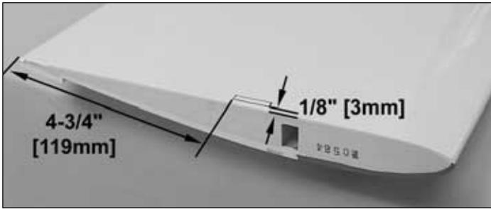
1. Use a hobby knife to cut a hole in the bottom of the wing sheeting for the **spoiler tubing** to exit the wing as shown.
