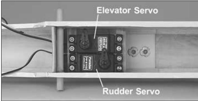
2. Install the servos using the hardware included with your radio system.
