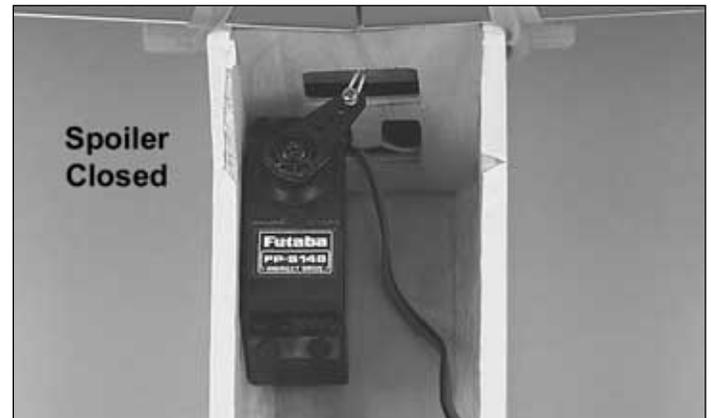
8. Mount the wing onto the fuselage and pull the ends of the spoiler strings up to the spoiler servo. Position the spoiler servo horn at the rearward end of its swing and wrap one spoiler string around the screw in the horn. With the spoilers held closed, apply a drop of CA to glue the string to itself, forming a small loop. Remove that string and do the same steps to the other string. The two strings should be the same
