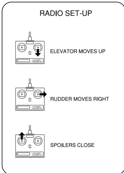
Use the sketch to make sure the control surfaces are moving the correct directions.
