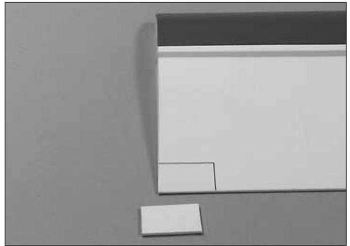
3. Mark and remove a small area of the covering on both wings for the 1/8" x 1" x 1-5/8" [3mm x 25mm x 41mm] plywood **trailing edge plates**. Glue the plates onto the wing with thick CA.
