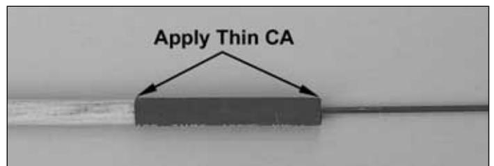
8. Use the **heat shrink tubing** at the end of the pushrod to hold everything in place as shown in the photo. Apply a few drops of thin CA to each end of the heat shrink tubing to secure it.
