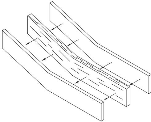
1. Use either epoxy or thick CA to glue one of the 1/16" [1.5mm] **aluminum joiners** to the 1/8" [3mm] **balsa joiner**. Apply as much pressure (clamps, clothes pins, weights, etc.) as possible while the glue is curing and be sure to line up the two pieces accurately. Glue the other 1/16" [1.5mm] aluminum joiner to the other side of the 1/8" [3mm] balsa joiner using the same procedure.
