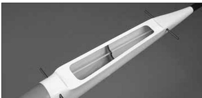
❑ 8. Glue the carbon fiber **wing dowels** into the fuselage with a small amount of thin CA. Be sure the length of the carbon on each side is equal.
