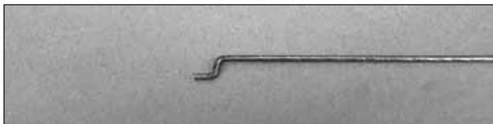
❑ 4. Locate the two 40" [1016 mm] pushrod wires. Put a Z-bend in one end of each wire as shown. Z-bend pliers work best for this.
