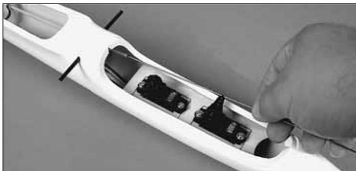
❑ 5. Insert each wire into the pushrod guide tubes in the fuselage.
