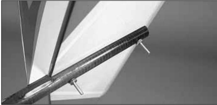
❑ 4. Secure the tail assembly to the fuselage using two #2 hex nuts and #2 flat washers as shown. Be sure not to overtighten the nuts as the stab could become damaged. Apply a drop of Threadlocker to each hex nut to prevent it from backing off.
