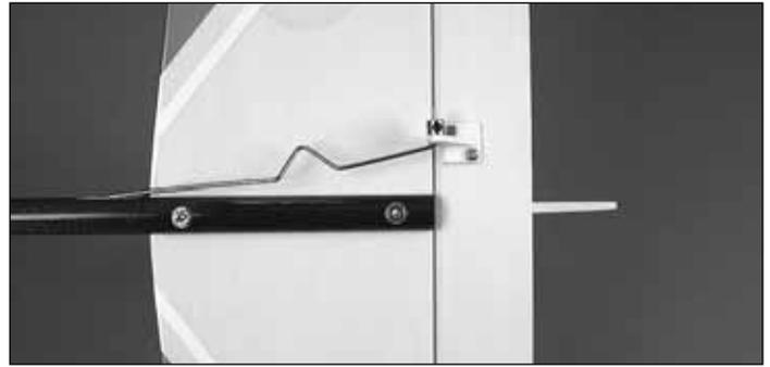
❑ 11. Attach the elevator control horn and pushrod the same way as the rudder control horn. The elevator control horn is positioned 1/4" [6.4 mm] from the fuselage boom as shown. Ensure that the holes in the control horn align with the hinge line.
