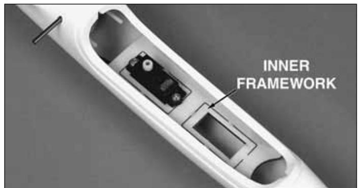
❑ 1. Install the servos in the **fuselage servo tray** as shown. If you will be using standard size servos, cut the inner framework away from the servo tray to accommodate these larger servos. **Note:** The following photos will show the installation of micro servos.
