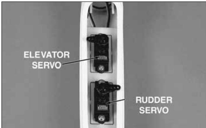
❑ 3. With the servos centered, install a servo arm onto each servo. Trim the arms as shown.
