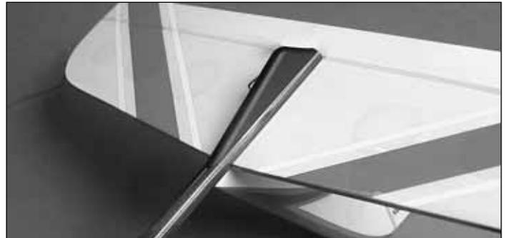
❑ 8. Insert the tail skid post into the slot cut in the tail of the fuselage and glue in place using CA as shown.
