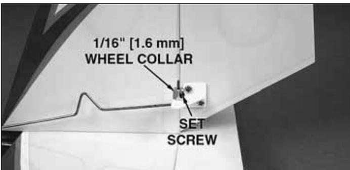
❑ 10. Slide a 1/16" [1.6 mm] wheel collar with set screw over the pushrod as shown. Secure the wheel collar by tightening the set screw. Add a drop of Threadlocker to the set screw to prevent it from backing out.
