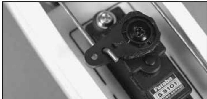
❑ 6. Remove the servo arms and insert the Z-bend into the second hole out from center on the arms. Reattach the servo arms and servo arm screws.
