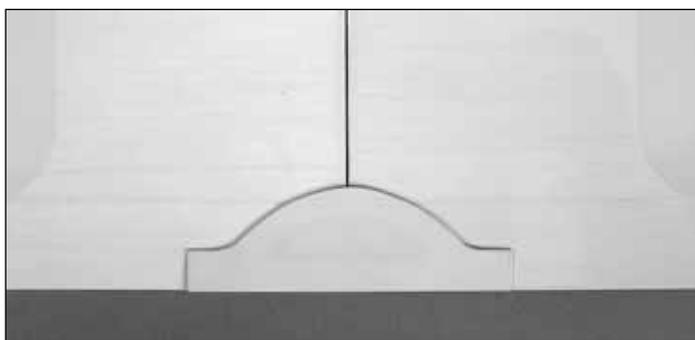
❑ 7. Glue the plywood **TE support** centered on the TE of the wing with CA.
