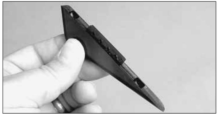
❑ 7. Glue the two tail skid pieces together as shown using CA.
