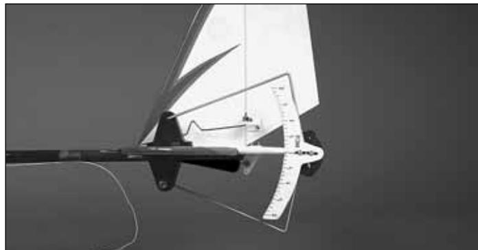
Use a Great Planes AccuThrow (or a ruler) to accurately measure and set the control throw of each control surface as indicated in the chart that follows. If your radio does not have dual rates, we recommend setting the throws at the **low rate** setting.
