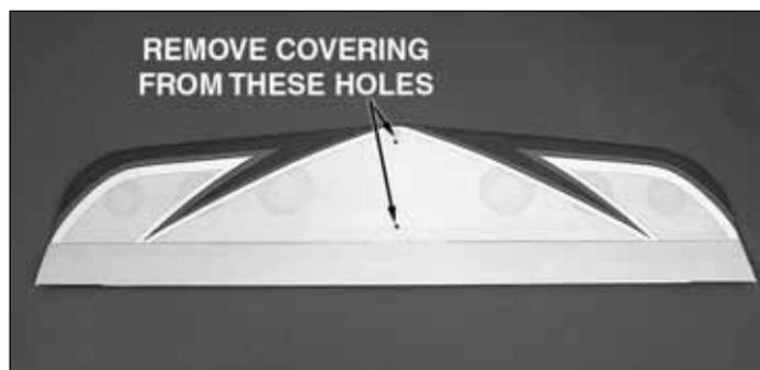
❑ 1. Locate the two small holes in the **stab**. Remove the covering from these holes using a sharp hobby knife.
