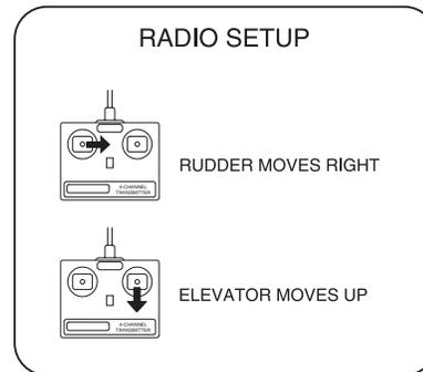
❑ 3. Make certain that the control surfaces respond in the correct direction as shown in the diagram. If any of the controls respond in the wrong direction, use the servo reversing switch in the transmitter to reverse the servos connected to those controls. Be certain the control surfaces have remained centered. Adjust if necessary.
