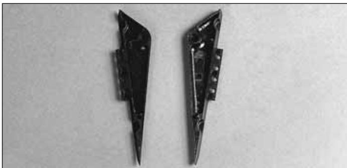
❑ 6. Locate the two plastic halves for the **tail skid**.
