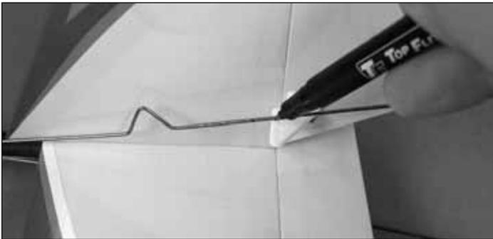
❑ 9. Make a mark on the pushrod where it crosses the control horn. Make a 90° bend at this mark and insert the pushrod into the second hole on the control horn.
