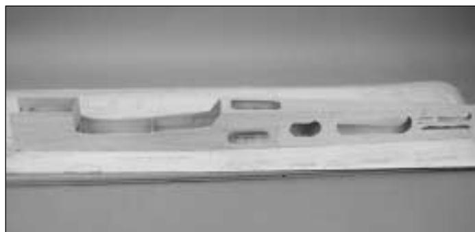
❑ 15. Fit the fuse sides and die-cut 1/8" balsa **fuse bottom** in place.
