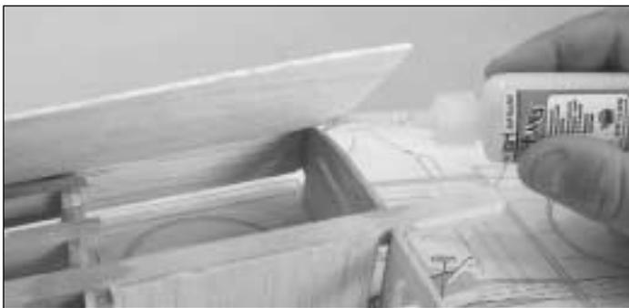
☐☐ 24. Being careful to keep the spar against the building surface and the ribs on the wing jig, use medium or thick CA to glue the sheeting to the ribs and the front half of the spar.
