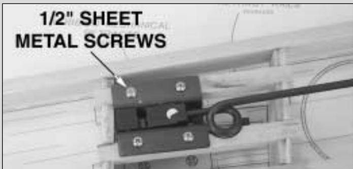
16. Place your retract in place on the rails. Drill four 5/64" pilot holes through the bass rails, using the mounting holes as a guide. Mount the retract with four #4 x 1/2" sheet metal screws (not provided).
