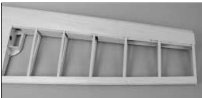
❑ 12. Using the 1/16" x 1/4" x 30" balsa sticks, cut, fit and glue **cap strips** to all of the exposed ribs, both top and bottom.
