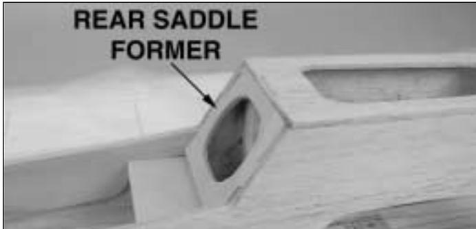
20. Sand a taper on the bottom edge of the die-cut 1/8" ply **rear saddle former**. Fit it in place, adjusting the taper until a good fit is achieved. Glue the former in place.
