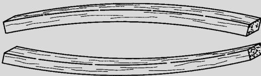
**TWO WARPED SPARS INSTALLED
