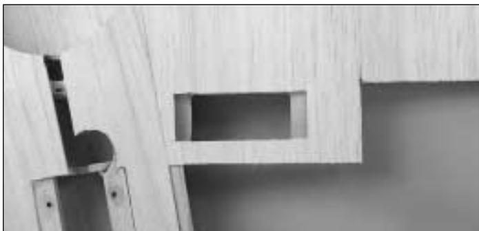
❑ 10. Cut openings in the bottom sheeting for the aileron servos.
