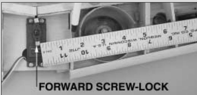
□ 7. On the left wing half, mark on the wheel well and rib 2A where a line from the **forward** screw-lock to the control link on the left retract intersects the wheel well and rib 2A.
