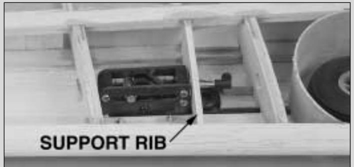
□ □ 37. Epoxy the die-cut 1/8" ply **retract support rib** in place.
