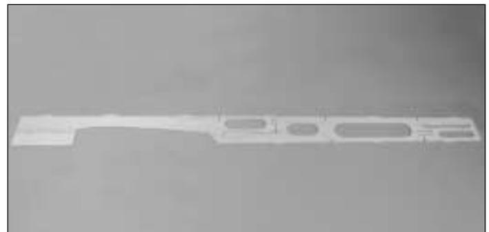
❑ 8. Cover the fuse side view of the plans with Great Planes Plan Protector. Fit and glue the die-cut 1/8" balsa **forward, center and fuse sides** together over the plan as shown in the photo.
