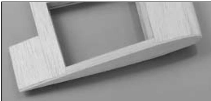
23. Cap both wing tips with leftover 1/16" balsa sheet. Sand to the shape of the wing.
