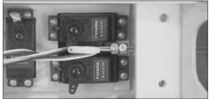
❑ 12. While keeping both elevators centered, connect the two elevator pushrods to each other with two 5/32" wheel collars and 6-32 x 1/4" hex head cap screws as shown in the photo. We recommend using thread locking compound on the cap screw threads.
