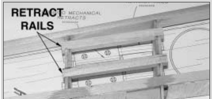
□ □ 14. Epoxy the two 1/4" x 3/8" x 4" basswood **retract rails** to ribs 3 and 4.
