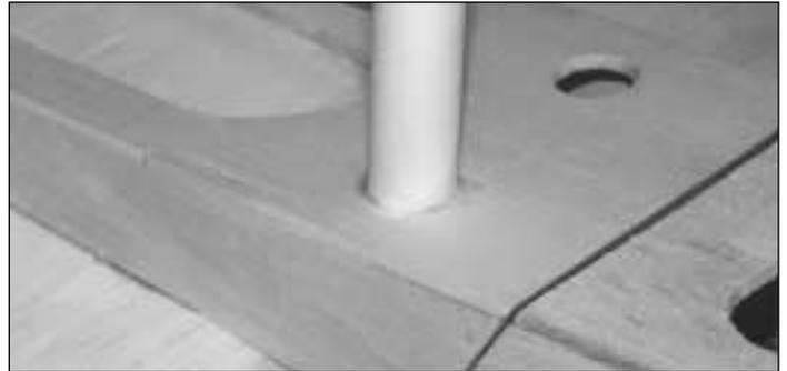
❑ 10. Mount the wing to the fuse with both wing bolts. Fit the **paper tube** through the belly pan bottom and around the head of the right wing bolt, flush against the wing bolt plates. Glue the paper tube to the belly pan bottom and wing bolt plate with medium CA. **NOTE:** Be careful not to glue the wing bolts to the wing.
