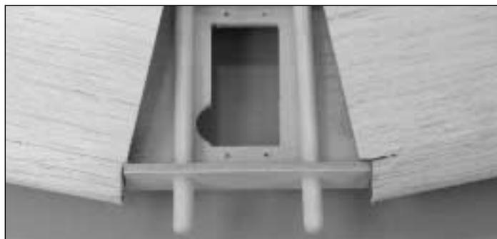
❑ 16. Trim the ends of the shaped LE so the forward dowel support will fit flush against the inboard ends of the LE and tight against the retract servo tray.
