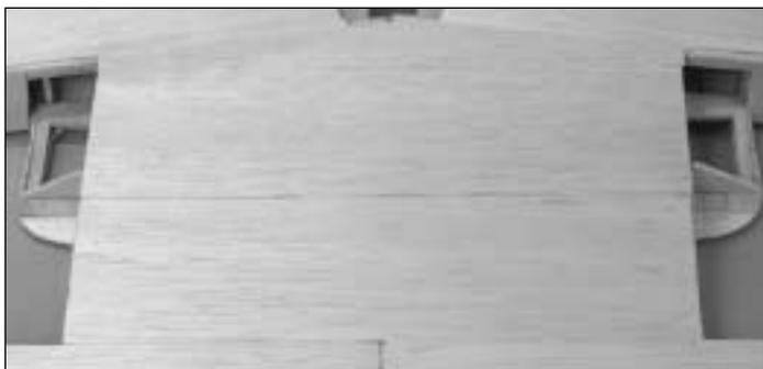
❑ 11. Use two 1/16" x 3" x 30" balsa sheets to sheet the top center section of the wing.
