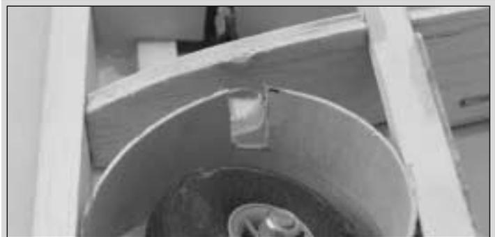
□ 8. Cut 3/8" wide by 5/8" deep slots in the outside edges of both wheel wells centered on the marks you made in steps 5-7.
