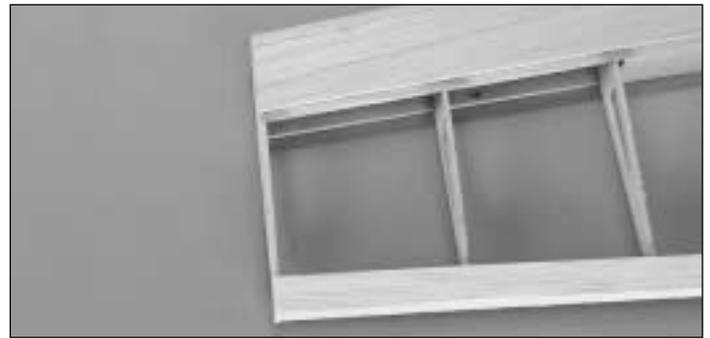
☐☐ 28. Trim the TE sheet, TE, LE, LE sheet and the spars flush with rib 9.
