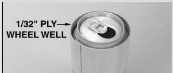
☐☐ 32. Select or cut a piece of 1/32" x 2" x 8-3/4" ply (not included) with the grain running the short way. Wrap it around a soda can of your choice, allow the sheet to overlap and glue the sheet to itself. This will be the wheel well.
