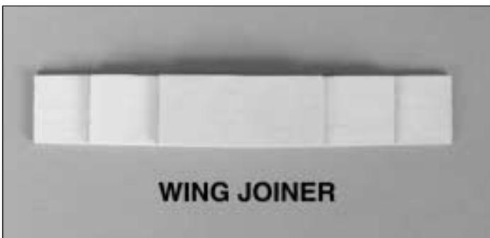
❑ 1. Using medium CA, laminate the three die-cut 1/8" ply **center spar joiners**. This complete assembly is now called the **wing joiner**.
