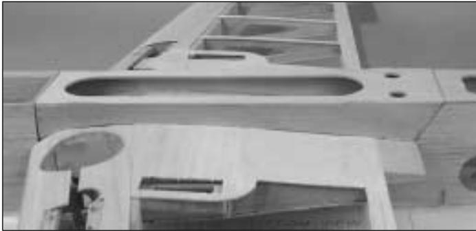
❑ 4. Now that the wing is accurately positioned, fit the belly pan to the fuselage tightly against the wing. When it is positioned and fitted properly, use a few drops of thin CA to **tack** glue the belly pan sides to the wing. Be careful to neither move the wing nor glue the wing or belly pan to the fuselage.
