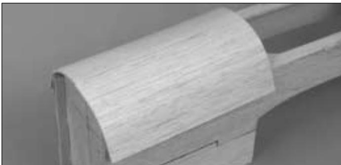
6. Wet the outside of the 5-1/2" x 6" sheet with water or a water/ammonia mix. Glue it to the firewall, instrument panel and stringers.
