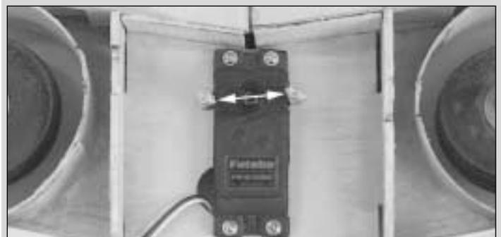
□ 10. Plug your retract servo into your receiver. Set it so that the servo arm, in the "up" position, is positioned rotated slightly as shown in the photo. Make sure it rotates clockwise to move the gear down.
