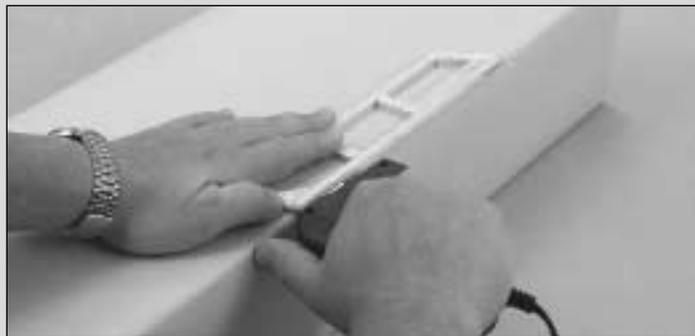
To cut the hinge slot, place the blades onto the wood where you want the slot. Lightly press the teeth into the wood. When you are satisfied with the location, press the button on the handle and the blades will cut easily into the balsa wood. Go to step 3 to complete hinging your stab.
