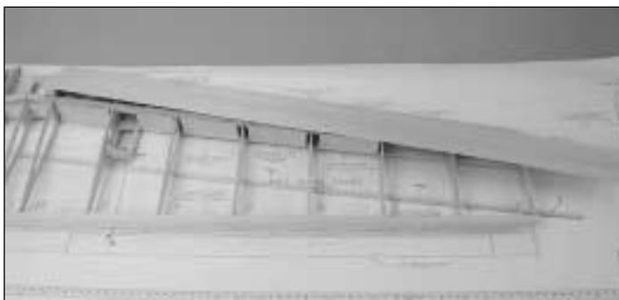
❑ 2. Edge glue a 1/16" x 3" x 30" sheet to the LE the same as you did for the bottom of the wing.
