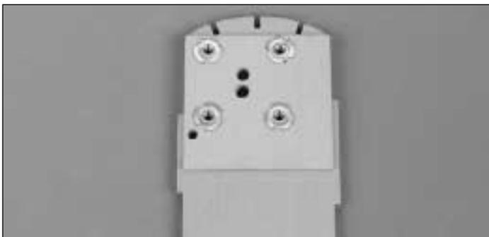
❑ 5. Press the four supplied 6-32 blind nuts into the holes on the back of the firewall. Gently tap the blind nuts with a hammer to fully seat them into the firewall, then add a few drops of thin CA around the blind nuts to secure them.
