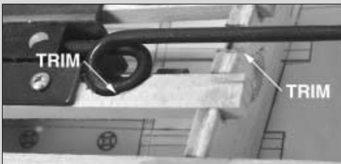
17. Remove the area of the rear landing gear rail that makes contact with the coil of the retract. Do the same where the strut makes contact with rib 3. **Hint:** Your rotary tool works well for both these tasks. Just be careful not to accidentally over trim.
