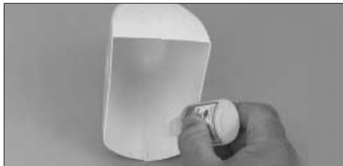
❑ 5. Glue leftover plastic strips to both halves overlapping the center joint.
