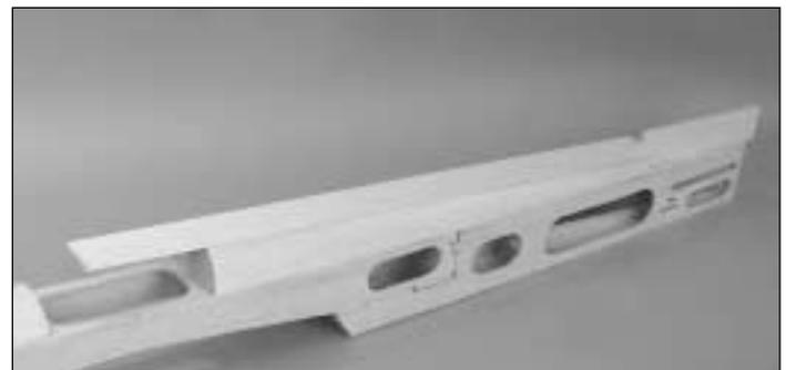
19. Glue the remaining 1/4" x 1-3/4" x 28" balsa **turtle deck top** to the top of the turtle deck sheeting and the tops of the formers. **Note:** Do not glue it to the fin filler block.
