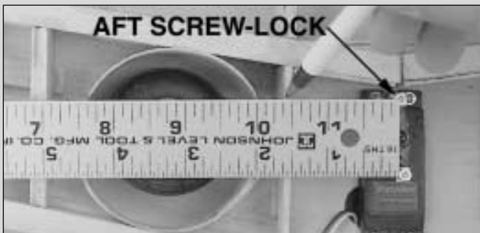
□ 6. On the right wing half, mark on the wheel well and rib 2A where a line from the **aft** screw-lock to the control link on the right retract intersects the wheel well and rib 2A.
