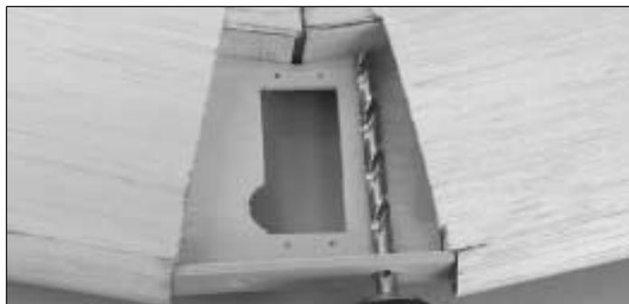
❑ 18. Remove the dowels and drill 1/4" holes through the 1/16" balsa shear webs.
