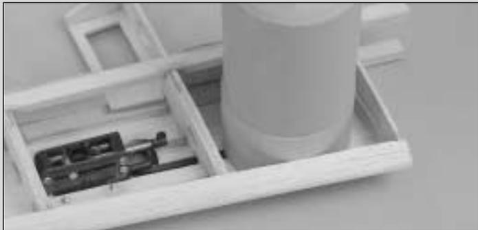
□ □ 33. Shape one end of the wheel well so that when slid in place it makes contact with the sheeting all the way around.
