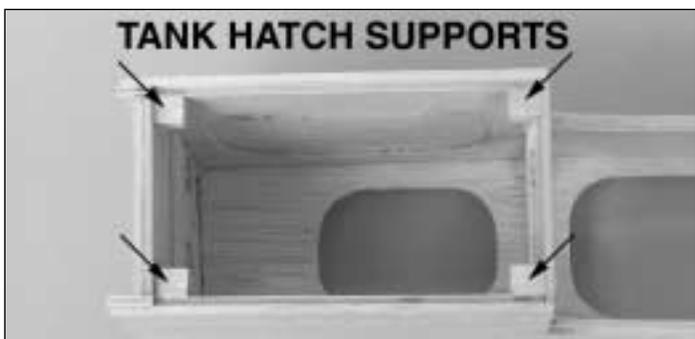
❑ 13. Glue one tank hatch support in each corner of the tank compartment, aligned with the bottom edge of the fuse doubler.
