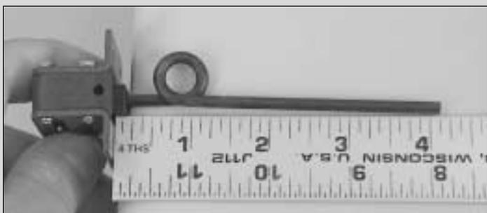
15. Using a rotary tool and a cutoff wheel, cut both retract struts so they are 4-1/8" long, measuring from the mounting plate on the retract body.
