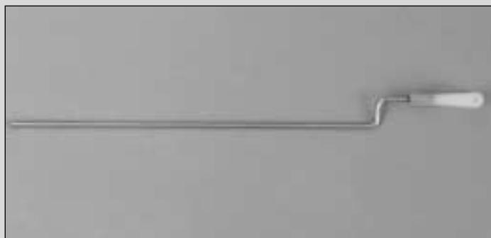
❑ 4. Cut 5/8" of the threads off the end of two 12" pushrods with clevises attached (GPMQ3772, not included). Bend to the shape as shown on the plans.
