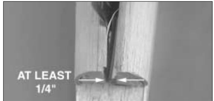
17. Trim the aft end of the 1/8" x 1/4" top stringers so there is at least a 1/4" gap between them, allowing sufficient space for the fin.
