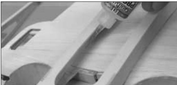
❑ 5. Remove the wing from the fuselage. Use medium CA to glue the rest of the belly pan to the wing at all contact points. **HINT:** Applying the CA from the inside of the belly pan helps minimize excess CA outside of the belly pan which would have to be sanded.
