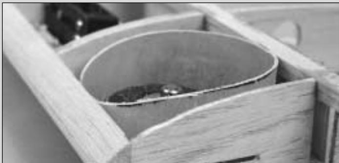
□ □ 35. Double-check the shaping of the well by looking at it from the inboard end of the wing. When satisfied with the fit, glue it to the sheeting, centering it between ribs 3 and 4. **Note:** Leaving the can in the well will help the well hold its shape as it is being glued.
