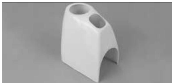
❑ 5. Use your hobby knife or a rotary tool with a sanding drum to clean up the crankshaft opening and air inlet.
