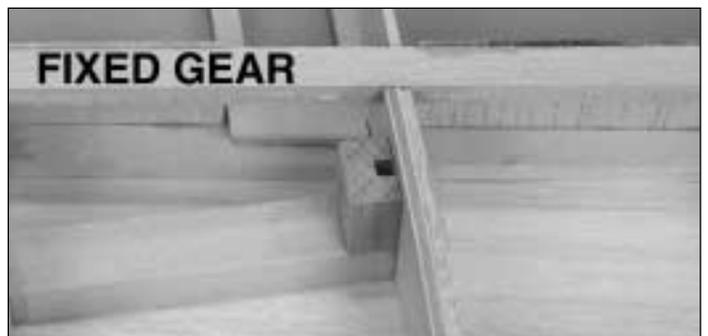
□ □ 38. If you are installing fixed gear, turn your wing right-side-up and epoxy the 7/16" x 5/8" x 3/4" maple grooved **torque block** to the rib 3 doubler and the landing gear rail, with the groove facing the doubler as shown in the photo.
