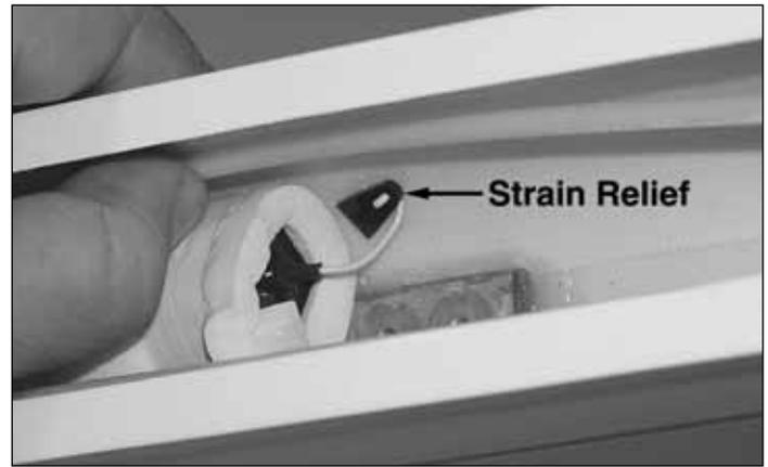
❑ 3. Drill a 1/16" [1.6mm] hole through the fuse side for the antenna. Take a cut-off piece of servo arm with at least two holes in it, and feed the antenna through two of the holes, making a strain relief which protects the antenna from accidentally being torn out of the receiver. Position the strain relief so that there is a small amount of slack between the receiver and the when the strain relief is positioned against the inside of the fuse.
