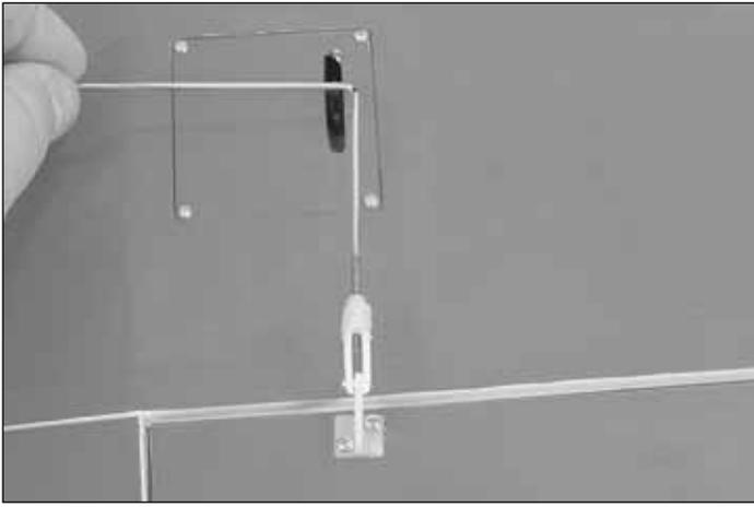
12. Attach the aileron clevis to the outer hole on the control horn. With the servo and aileron centered mark the location the pushrod crosses the servo arm. Bend a right angle in the pushrod at the mark.
