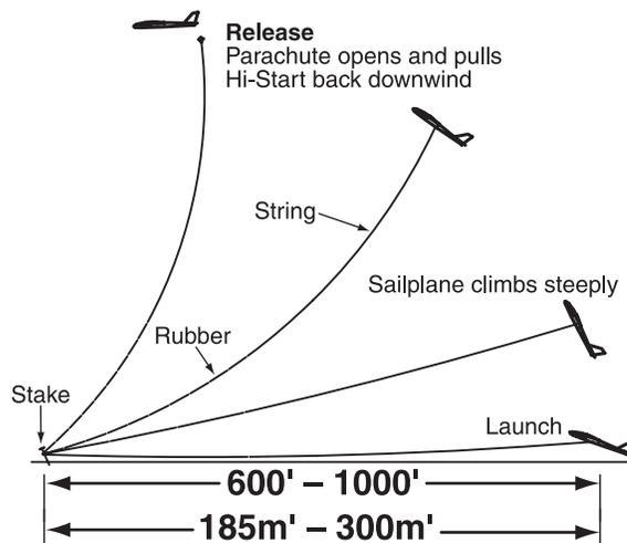
A hi-start is the most common way to launch your Spirit 100 ARF. Follow the directions that came with the hi-start and lay it out directly into the wind. Place the stake at the far upwind edge of the flying field so the parachute will blow back onto the flying field.
