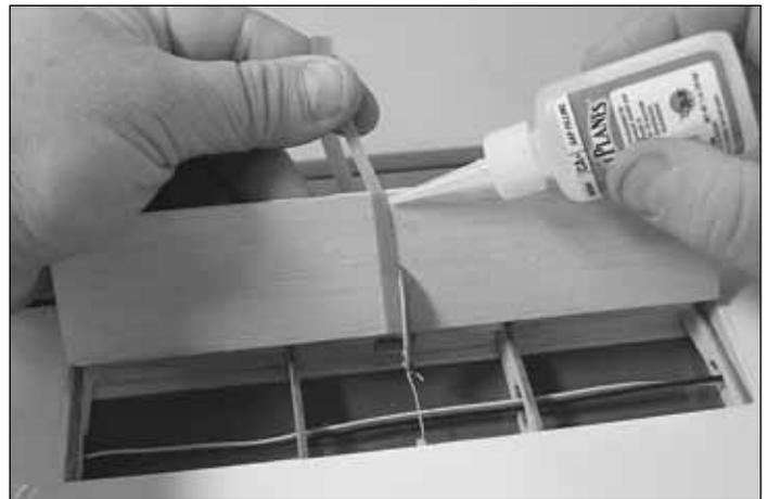
☐☐ 6. Pull the rubber band up the spoiler and glue near the TE with a drop of medium CA. **NOTE:** There should be just enough tension to close the spoiler.
