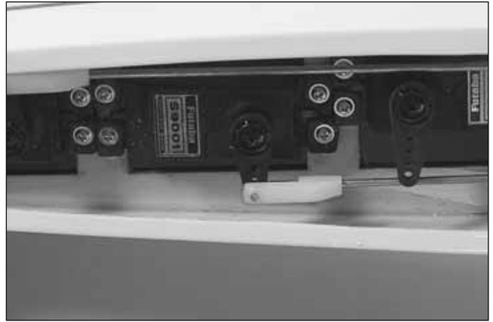
❑ 7. Attach the pushrod to the servo arm with a Faslink. Trim the excess pushrod from flush with the Faslink.
