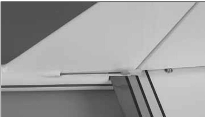
❑ 6. If necessary, bend a slight angle in one of the pushrods 6" [150mm] from the end of the clevis. Slide this pushrod into the rudder pushrod tube.
