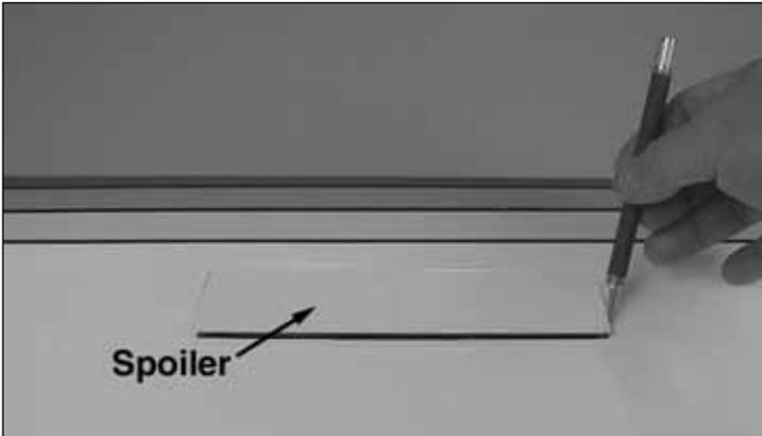
☐☐ 2. Trim the covering around the ends and TE of the spoiler. DO NOT cut the along the LE
