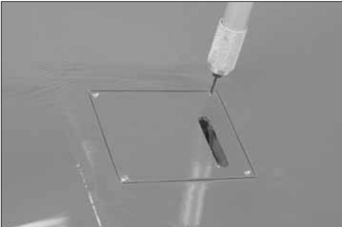
❑ 7. Attach the servo lead to the extension. Fit the servo hatch to the wing. Use the holes in the cover as a guide and drill four 1/16" [1.6mm] holes through the plywood servo hatch mounts.
