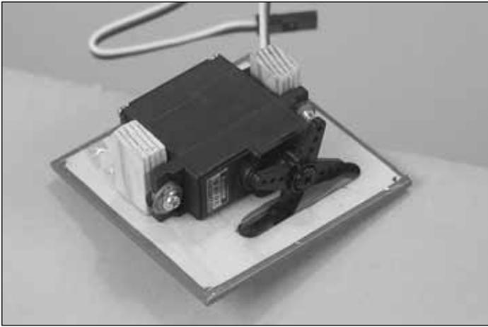
❑ 6. Attach the servos to the blocks using the hardware that comes with your radio system. **HINT:** Drill a 1/16" [1.6mm] pilot hole for the servo screws and strengthen the holes with a drop of thin CA.
