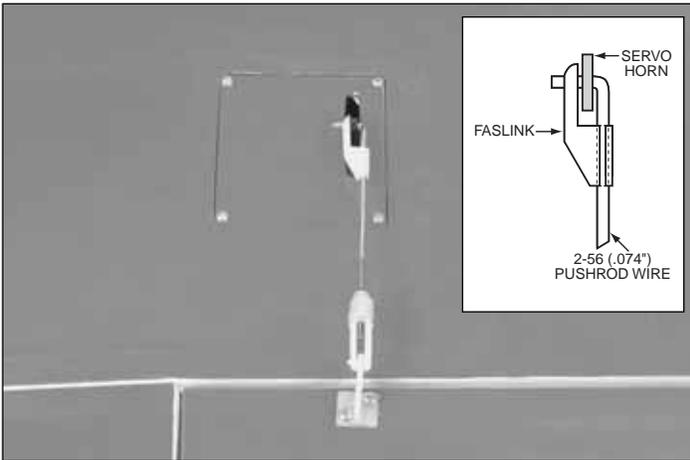
13. Cut the pushrod 1/4" [6mm] past the bend. Push the pushrod through the servo arm. Retain the pushrod with the nylon faslink.
