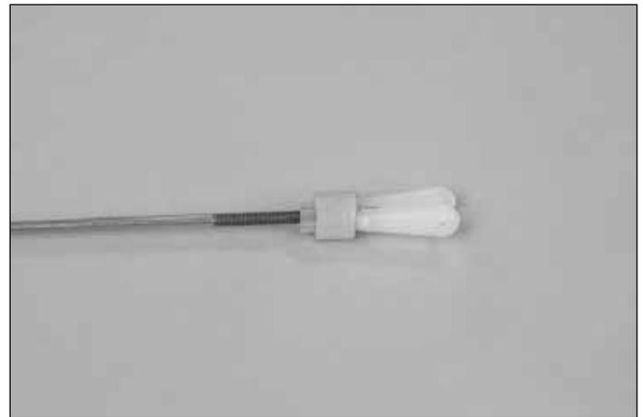
❑ 11. Screw a nylon clevis 15 turns onto each of the four 12" [305mm] pushrods. Slide a silicone retainer on each of the nylon clevis.
