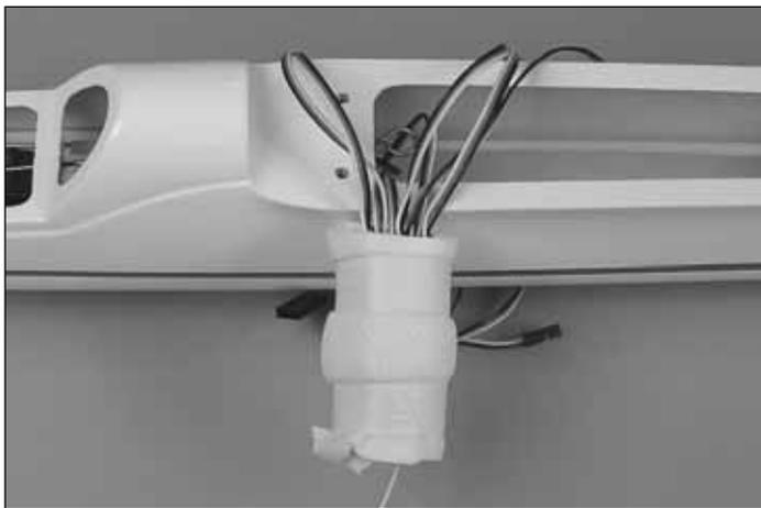
❑ 1. Attach the switch, charge jack, servos and servo extensions to the receiver. Wrap the receiver in foam.
