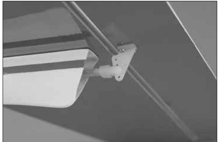
❑ 9. Slide the second 42" [1067mm] pushrod into the elevator pushrod tube from the rear.
