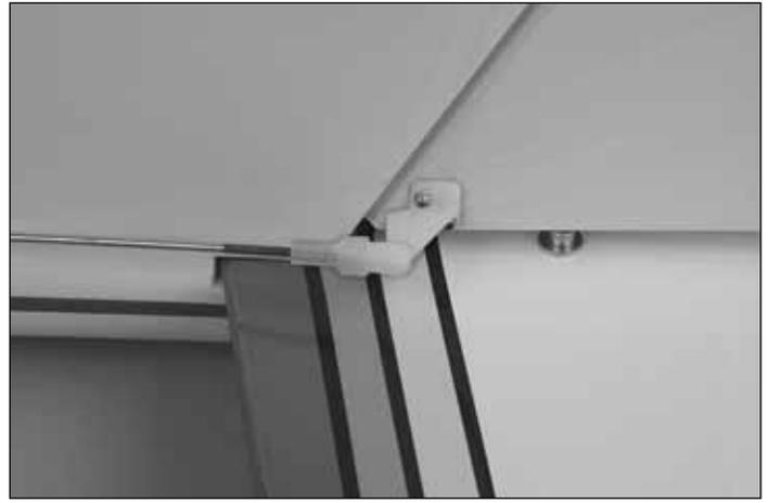
❑ 7. Align the rudder control horn with the rudder pushrod. Glue the control horn to the rudder with a small drop of CA.
