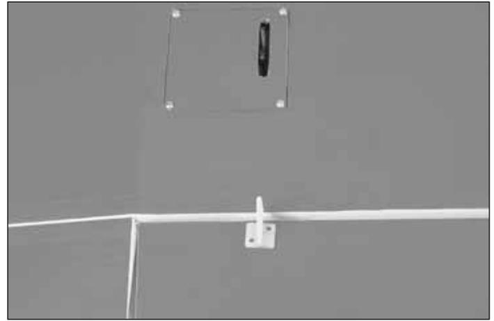
❑ 9. Align the aileron control horn with the servo arm. Glue the control horn to the aileron with a small drop of CA.
