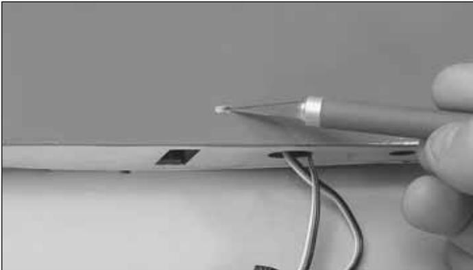
☐☐ 3. Trim covering from the spoiler string tube on the bottom of the wing.
