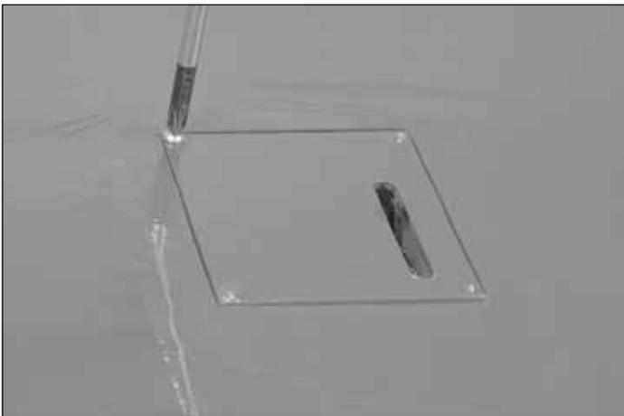
❑ 8. Temporarily mount the servo hatch cover to the wing with four #2 x 3/8" [9.5mm] screws. Remove the screws and hatch. Then, harden the holes in the wing with thin CA. Allow the glue to dry and remount the servo hatch cover.
