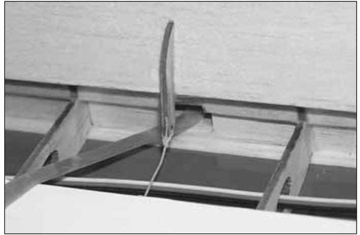
☐☐ 5. Cut a #64 rubber band in half. Clean the rubber band with alcohol. Glue one end of the rubber band to the front sheer web with a drop of medium CA.
