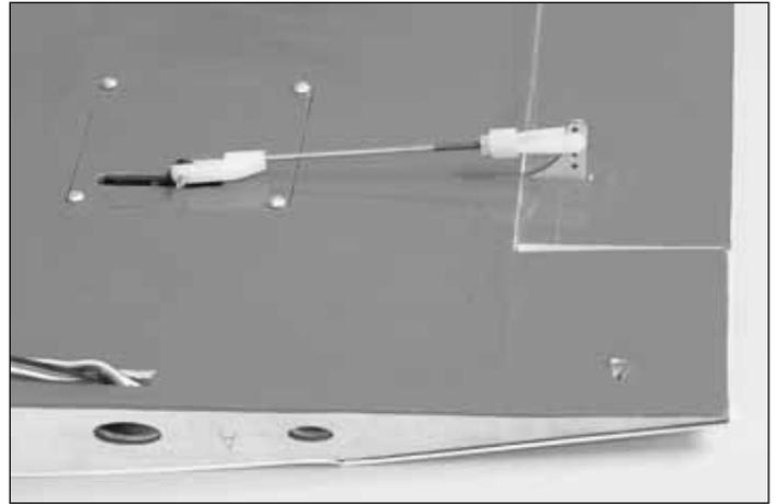
16. Cut the pushrod 1/4" [6mm] past the bend. Push the pushrod through the servo arm. Retain the pushrod with the nylon faslink.
