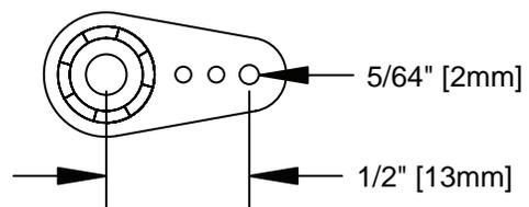
❑ 1. Make two single sided servo arms that have the outer hole 1/2" [13mm] from the servo mounting hole. Enlarge the outer hole with a 5/64" drill bit.
