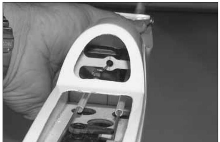
❑ 9. If you will be using spoilers slide the spoiler activation rod forward through the hole in the former at the front of the wing opening.
