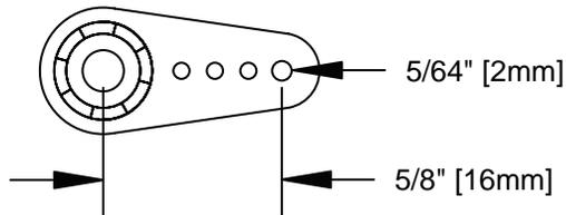
❑ 2. If you will be using the spoiler option make a servo arm that has the outer hole at least 5/8" [16mm] from the servo mounting hole. Enlarge the outer hole with a 5/64" drill bit.
