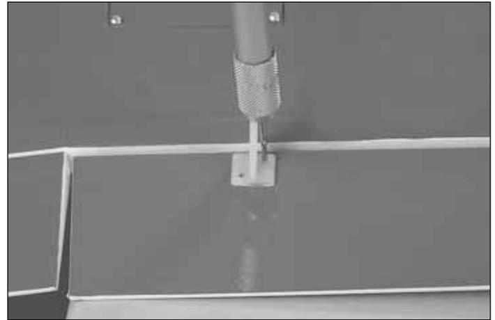
❑ 10. Drill two 1/16" [1.6mm] holes through the aileron. Secure the control horns with two 2-56 x 1/2" [13mm] screws and the nylon control horn back.
