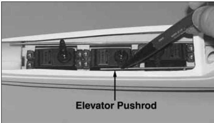
❑ 5. Center the elevator and mark the pushrod where it crosses the hole in the servo arm.
