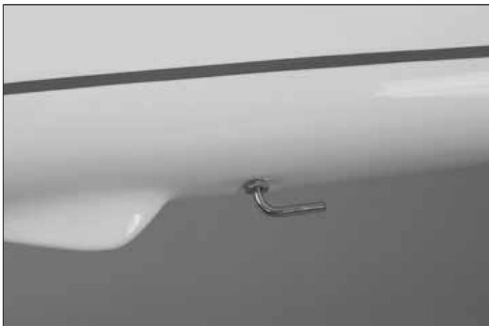
5. Mount the 6-32 tow hook to the fuse with the 6-32 nut to lock it in place.
