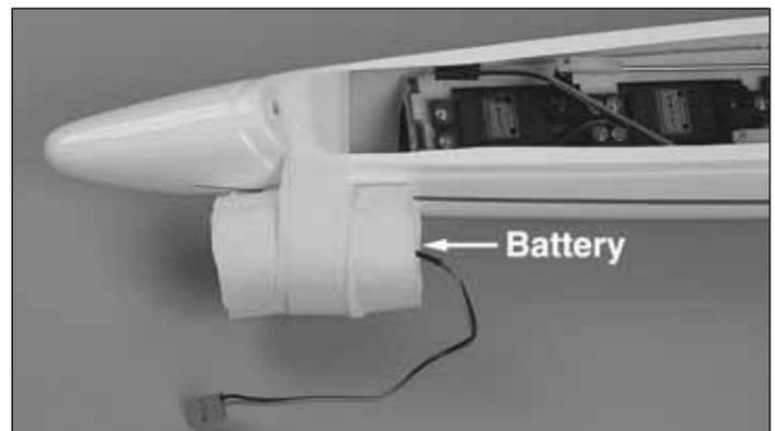
❑ 1. Wrap the receiver battery in foam and tape. Tape the battery to the outside of the fuse. **NOTE:** The battery will be installed after the CG is set.
