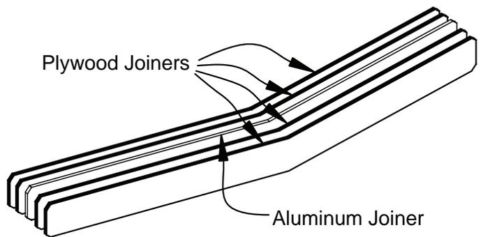
1. Make a sandwich of the wing joiners as shown in the sketch. Glue the wing joiners together with 6-minute epoxy and clamp together. Use a paper towel dampened with alcohol to remove the excess epoxy that has squeezed out of the joiners.
