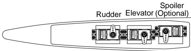
❑ 3. Mount the rudder and elevator servos with the hardware provided with the servos. If you will be using spoilers install the spoiler servo also. **NOTE:** The spoiler servo mounts as far right as it will go in the servo tray.
