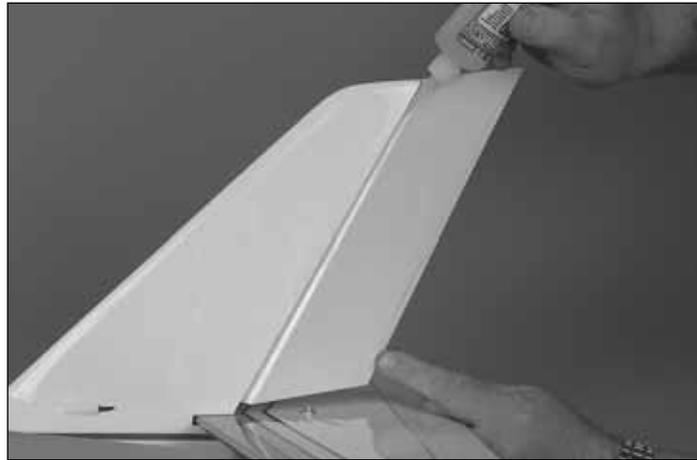
❑ 4. Fit the rudder to the fin with the hinges. Glue both sides of each hinge with 3 drops of thin CA.
