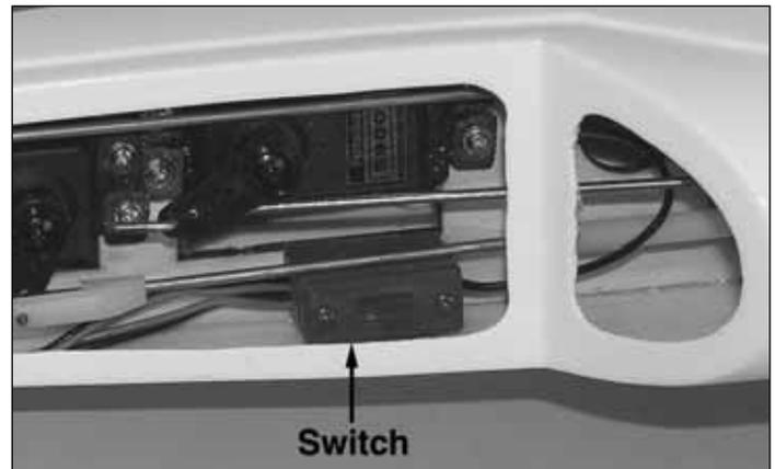
❑ 4. Mount your switch in the canopy area with silicone glue, making sure it does not interfere with the pushrods or canopy.
