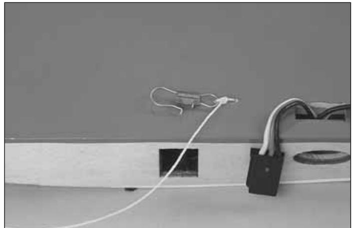
☐☐ 8. Pull the slack out of the spoiler string without opening the spoiler and tie the spoiler hook to the string so that the rear of the hook lines up with the front of the string opening.
