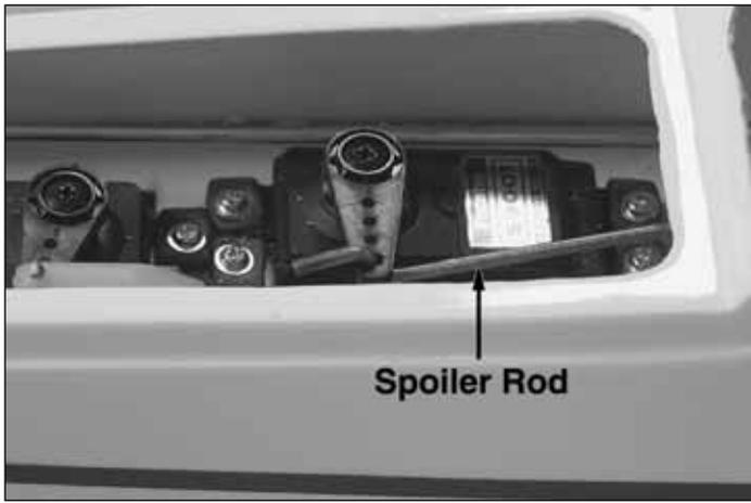
❑ 10. Attach the Z-bend end of the spoiler activation rod to the spoiler servo.
