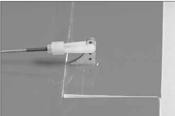
14. Harden the control horn with thin CA and drill out the second hole with a 1/16" drill. Attach the flap clevis to the second hole on the control horn.
