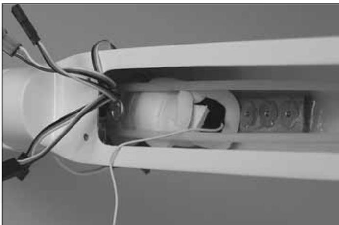
❑ 2. Push the receiver into the bottom of the fuse and retain it with a small piece of Velcro®.
