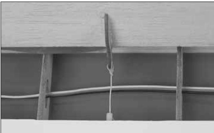
☐☐ 4. Insert the spoiler string in the string tube. Tie the end to the spoiler control horn and secure with a drop of thin CA.
