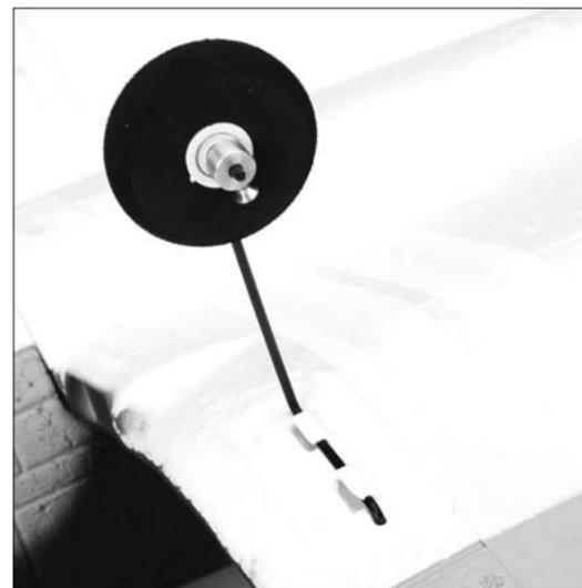
**NOTE:** The landing gear is directional. When properly installed, the landing gear will rake forward to add stability in landing. If the gear does not angle forward when installed, simply reverse the landing gear.
