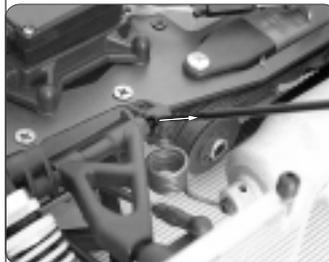
Caster angle is commonly adjusted with nylon spacers that are inserted either in front or behind the upper front suspension arm. More spacers in front will increase the caster angle, while more spacers behind will decrease the caster angle. On a carrier or kingpin-style steering system, caster is typically adjusted by changing the spindle carrier. To remove the nylon spacers use EXHAUST SPRING / CASTER CLIP REMOVER TOOL, part#10 7610.
