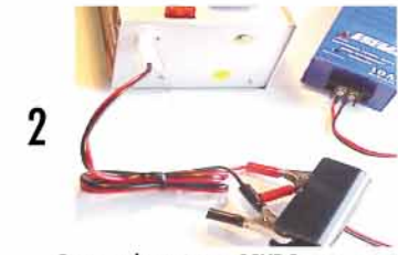
2 Connect the unit to a 12VDC power supply
