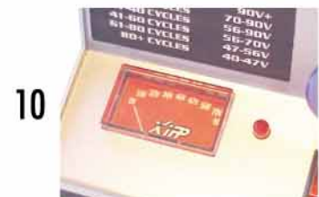
10 Meter should read zero and Xapping is completed If the meter is not at zero...DO NOT REMOVE the cell or touch copper terminals. Wait 5 min for self-discharge to zero V.
