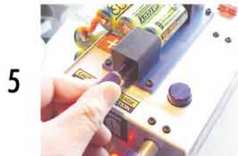
5 Tighten the + terminal copper contact
