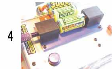
4 Install battery to cell holder (observe polarity)
