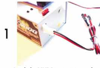
1 Attach the 12VDC input wiring to the unit
