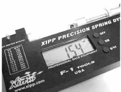
This spring provides 154g of tension
