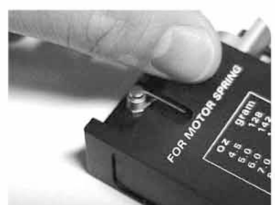
Apply tension until the spring lock it's end into the groove as shown
