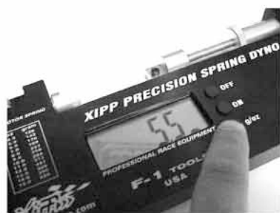
Switch the unit measurement and the spring dyno showing 5.5oz of pressure
