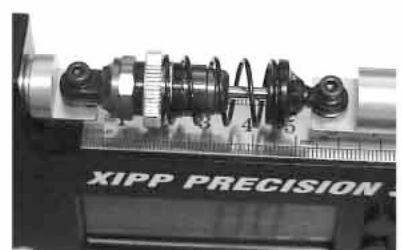
Remove any motor spring and you can test a suspension spring, this example shows a TC spring mounted using two 3mm screws
