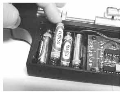
Install the AAA batteries by opening the back cover
