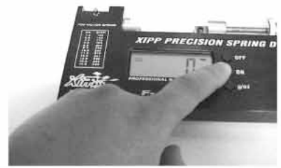
With no spring on the unit, turn it on and it will automatically zero itself
