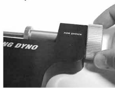
Compress the spring and lock the unit by turning the knob clockwise
