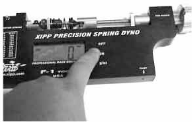
Zero the unit by pressing the "ON" button
