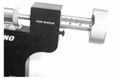
This time we use 30mm instead because the shock travel is much longer and we get a more accurate reading this way
