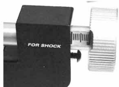
This picture shows the 10mm marking. At this point, your shock should move freely for at least 10mm of travel
