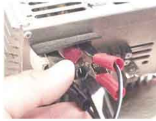
Connect Dyno to a 12VDC power source
