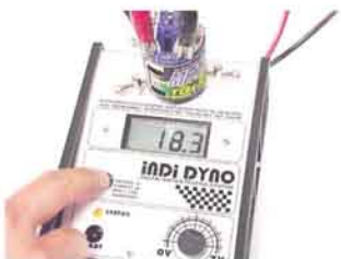
This motor has 18.3 interference index, which is pretty low for this type of motor
