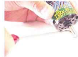
Tighten the coupling with a 1.5mm wrench
