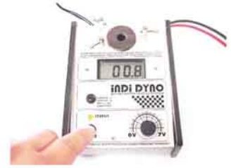
Press start & the status LED should be on
