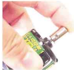
Insert the magnetic coupling
