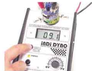
This motor draws 9.1 Amps during test
