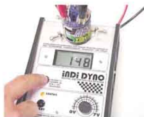
This motor is running at 14,800rpm
