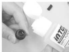
STEP5, Fill the main shock body with 100% silicone shock oil, make sure that there is no air bubble
