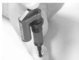
STEP8, Fully compress the shock shaft
