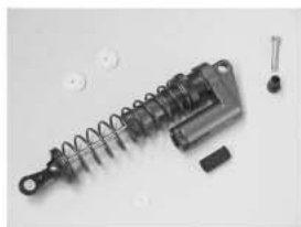
STEP1, These are all the parts for one shock, two pistons are extra
