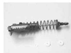
STEP12, One shock is now completed with spring and spring retainer
