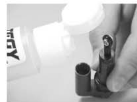
STEP9, Flip the piggyback over and fill it up at least half way
