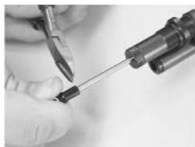
STEP3, Tighten the plastic rod end
