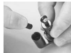
STEP11, Drop in the cylinder shape foam, add shock oil and close the bottom cap
