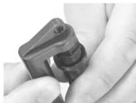
STEP7, Install the piggyback now but do not over-tighten the top cap
