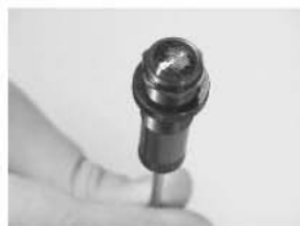
STEP6, Fill oil to the top and keep the shock body vertical. We suggest 35 to 45 weight oil
