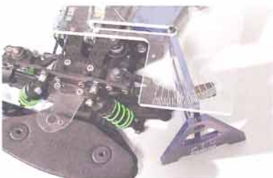
Check max steering angle
