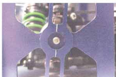
Align the castor gauge with the front kingpin using eyeball method
