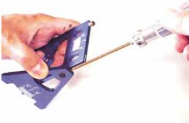
Lock the set screw as shown
