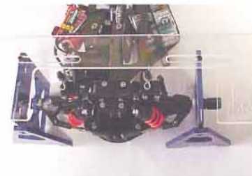
Ruler measures toe-in/out & steering angle
