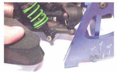
Front camber/caster at ride height
