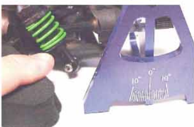
Check front camber/caster at full suspension compression
