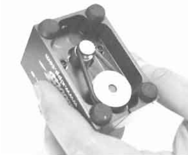
Install drive o-ring as shown
