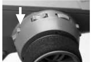
The brake trim allows you to adjust the lock point by 7 increments in each direction. Each increment offsets the lock point by at least 1% (fine) and at most 10% (coarse). You can select the size of the trim increments in the menu point „STEP“ of the „
