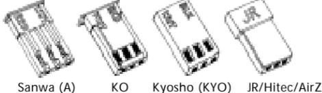
**FIGURE 1** With a small standard screwdriver, press on each of the three metal prongs until the wires are easy to remove. Remove wires.
