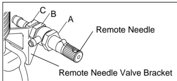
Connect the needle-valve to carburettor jet nozzle with silicone tubing supplied. In the event of the tubing becoming damaged, it should be replaced with 78mm length of 5mm ODx2mm ID silicone tubing.
