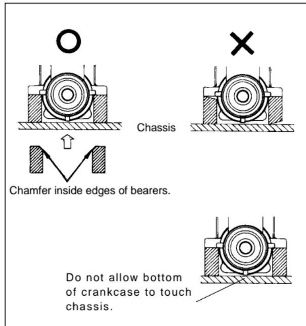
Avoid forcing the screws. Secure with locknuts. If the bottom of the recoil starter housing touches the car chassis, install the engine mount spacers (supplied) between the engine's mounting lugs and the engine mount. Use the M3x15 screws provided. With some vehicles, it may be necessary to make minor trimming modifications to chassis or body when fitting the engine.
