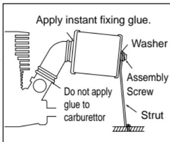
2. Fit the other end of the elbow over the carburettor intake and secure with strap supplied. Do not use glue at this point.
