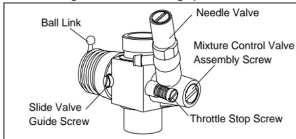
**NOTE: Readjustment may be necessary, occasionally to allow for changes in fuel formula, gear ratio or clutch engagement point.**
