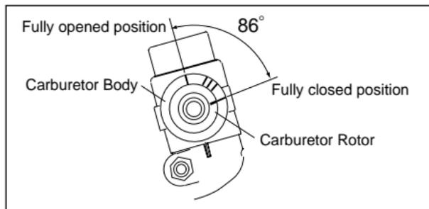
As shown in the sketch, the carburetor has graduation marks. When the triangle mark on the carburetor rotor meets the far right mark, the throttle is fully closed. When the triangle mark meets the top mark, the throttle is fully open. The range is 86 degrees. You may use the other three marks as the reference marking of throttle opening to your preference when hovering.
