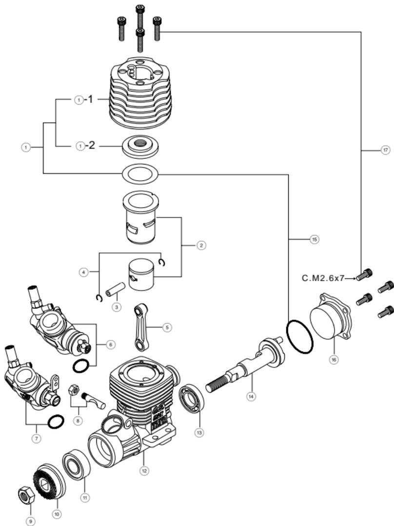
\* Type of screw C··Cap Screw M··Oval Fillister-Head Screw
