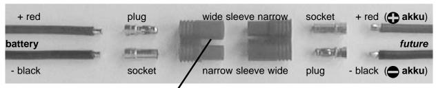
**Caution:** remove locating lug from battery cable. Do not remove lug from any cables attached to controllers or charge leads!
