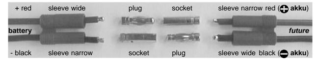
Fit the connectors in the order shown above; the contacts are pressed in as follows:
