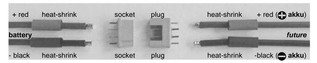
**Fit** the connectors in the order shown above; the contacts are soldered as follows:
