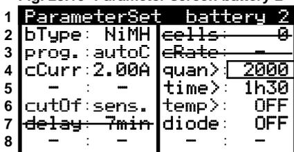
Fig. 23.11 charge quantity selection b.2
