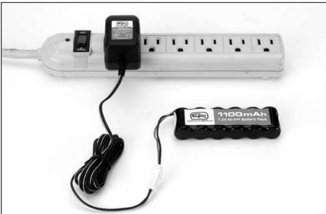
Plug the AC charger into the proper wall receptacle (110V). Plug the battery pack into the charger and let it charge for 3 hours for the first time. After running, or when your Tailwhip slows noticeably, recharge the battery pack for 5–6 hours for a full charge.
