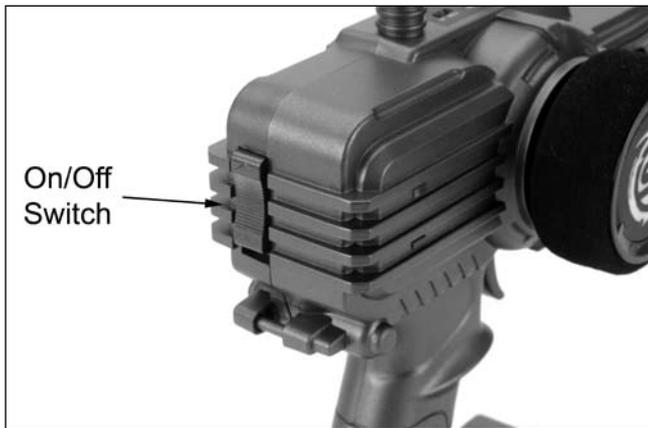
Always turn on the transmitter first by sliding the switch on the left side of the wheel from bottom to top. The small red and green lights above the switch should both light up. If not, you need to check for low or incorrectly installed batteries.
