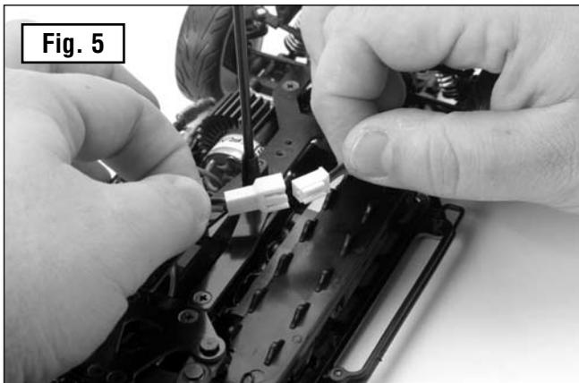
Once the battery is charged, remove the body clip from the front battery post (Fig. 3) and insert the battery in the clear Lexan battery holder (Fig.4). Reinstall the battery clip and plug the battery into the ESC.
