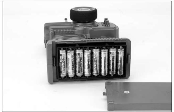
Remove the transmitter battery cover by sliding the cover from left to right. Install eight (8) AA batteries into the battery holder. Pay close attention to the correct direction of the positive (+) and negative (-) ends as marked in the tray. Once all 8 batteries are in place, reinstall the battery cover by sliding it on from right to left.
