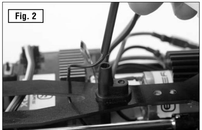
Insert the antenna wire through the antenna mount and into the antenna tube (Fig.1) pushing it through until it comes out the other end. Push the antenna tube (Fig. 2) into the antenna mount.
