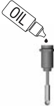
4 Push the shaft up until the piston is level with the top of the body. The oil will bulge up above the shock body.
