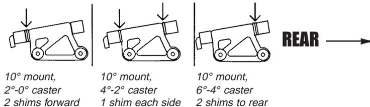
example would be a starting caster of 2° will have 0° caster at full suspension travel and a starting caster of 6° will be only 4° at full suspension travel.
