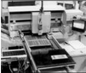
Ultra-precise, high-density, computer controlled, automated assembly machines ensure that you get consistent high quality.
