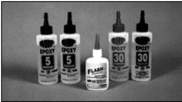
**Adhesives** - You will need two types of adhesives for this ARF - Epoxy and Instant (cyanoacrylate) adhesives. We recommend that you purchase both 5-minute and 30-minute epoxy to cut down on assembly time, but you can get by with only 30-minute epoxy if time is not important. You will also need a small bottle of both "Thick" and "Thin" instant adhesive.
