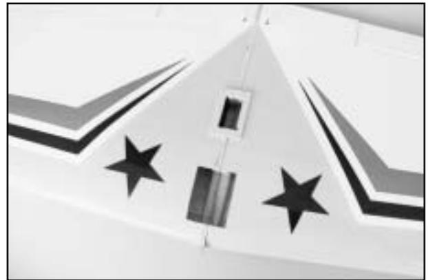
❑ Cut away the balsa sheeting to expose the retract servo location. Also cut away for the aileron servo opening. Glue the aileron servo tray in place, removing the covering film first.
