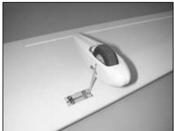
□ Locate the main landing gear and install them into the slots/holes in the landing gear blocks. Secure with metal landing gear straps and screws. Pre-drill the screw holes with a 1/16" bit.
