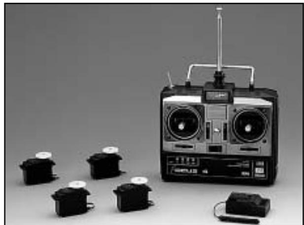
**Radio** - A 4-channel radio with four standard servos is required. (If you are installing retracts, you need a radio that has at least 5 channels and a 180° Retract Servo that is compatible.)
