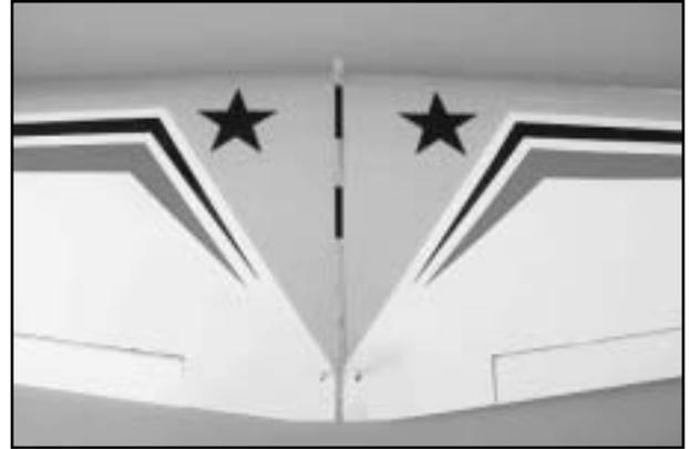
❑ Epoxy the wing halves together, making sure you coat all sides of the dihedral brace plus where the ribs join. Use some masking tape to hold the wing together as the glue sets.
