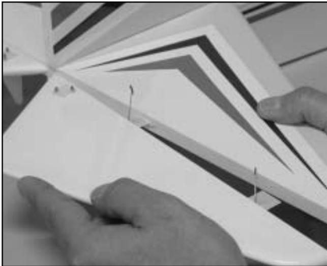
□ With the C.A. hinges in place on the elevators use a small T-pin to hold the hinge in place when installing onto the stabilizer. Apply a small amount of thin C.A. to all 4 hinges, remember to apply glue to the top and bottom of the hinges.
